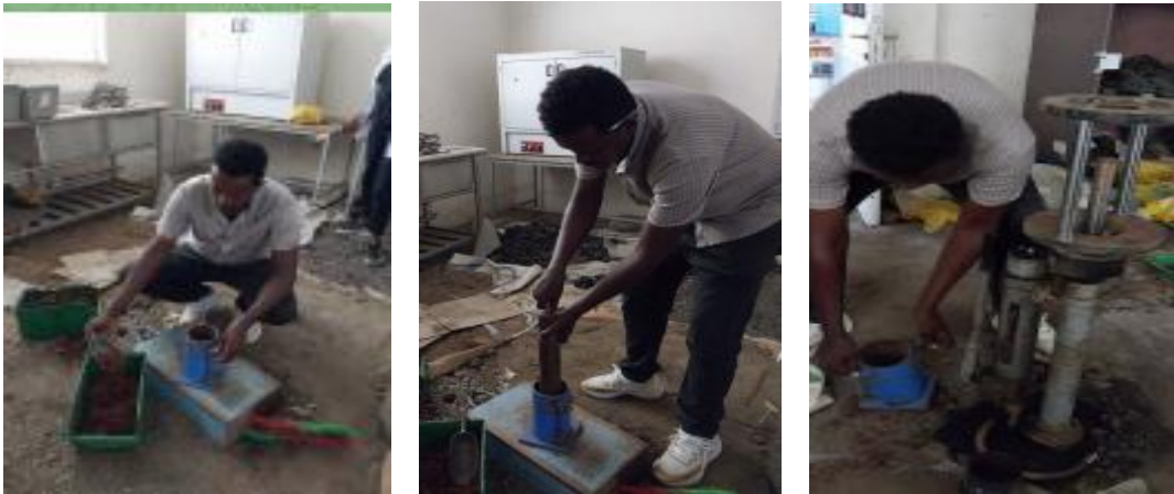
Figure 3.7 Compaction test procedure
