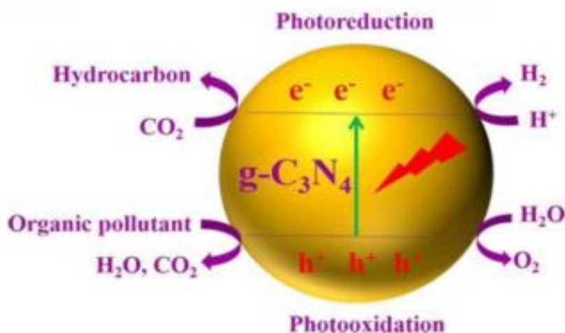
Figure 5. Photocatalytic degradation mechanism of g- C_3N_4 (Geo and Zhang, 2020)
