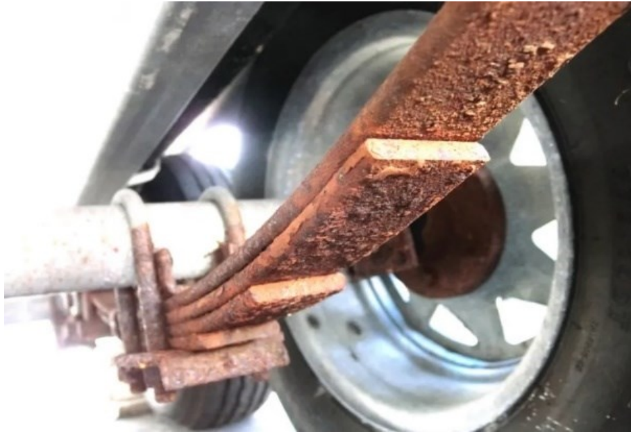
Figure 1.5: Corrosion in Traditional Leaf Spring (Fernie, 2016)
