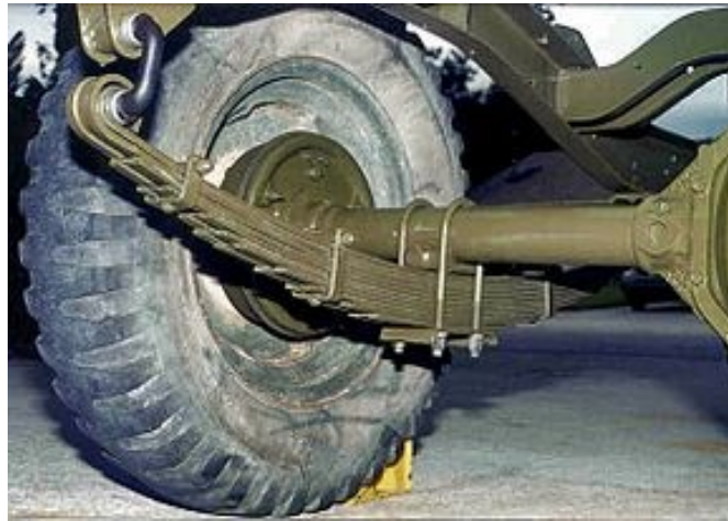
Figure 1.3: Conventional Leaf Spring on heavy duty vehicles (Batu et al., 2021).
