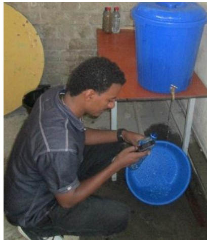
Figure 3.11: Measuring flow rate
