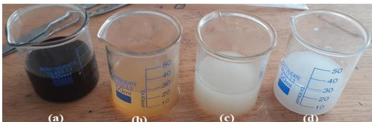
Figure 9. Testing of different concentrations of H_2SO_4 to obtain CNC without damaging the structural integrity of the cellulose. (a) 65%, (b) 55%, (c) 45% and (d), 35% of H_2SO_4 .
