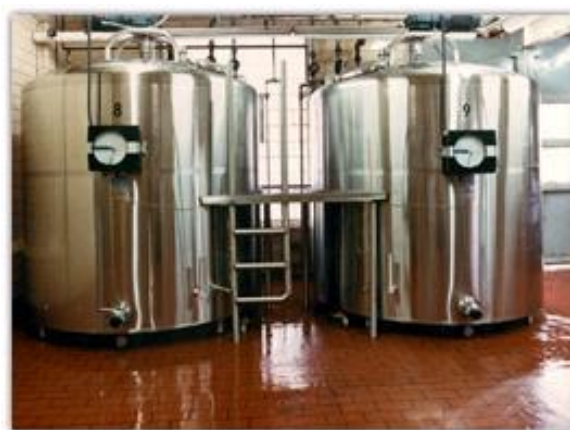
Figure 1.1 Chemical batch reactor tank (University of Michigan, 2022)
