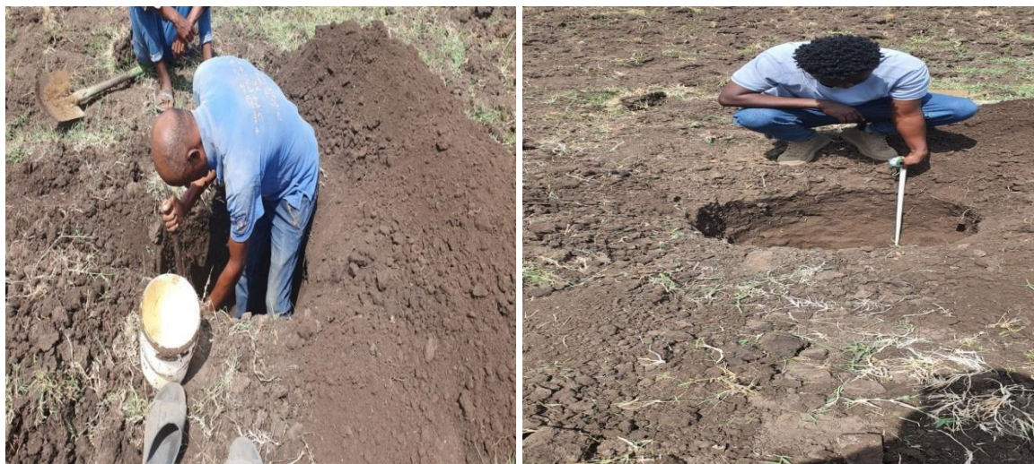
Figure 3. 2 Photographic view of expansive sample pit and disturbed soil sample
