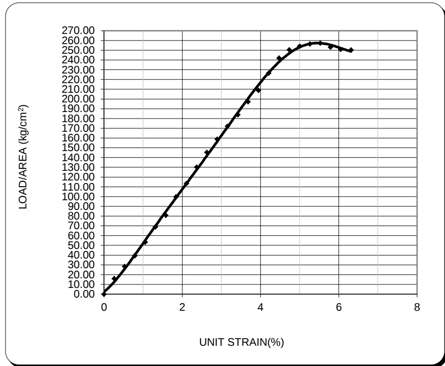
Figure C-20 UCS curve for soil sample 1(pit 1) and fly ash mix 60% E-40% F
