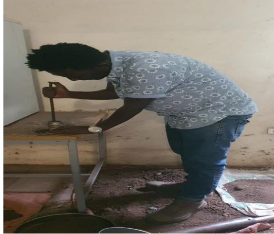
Figure 3. 5 Photographic view of UCS specimen preparation
