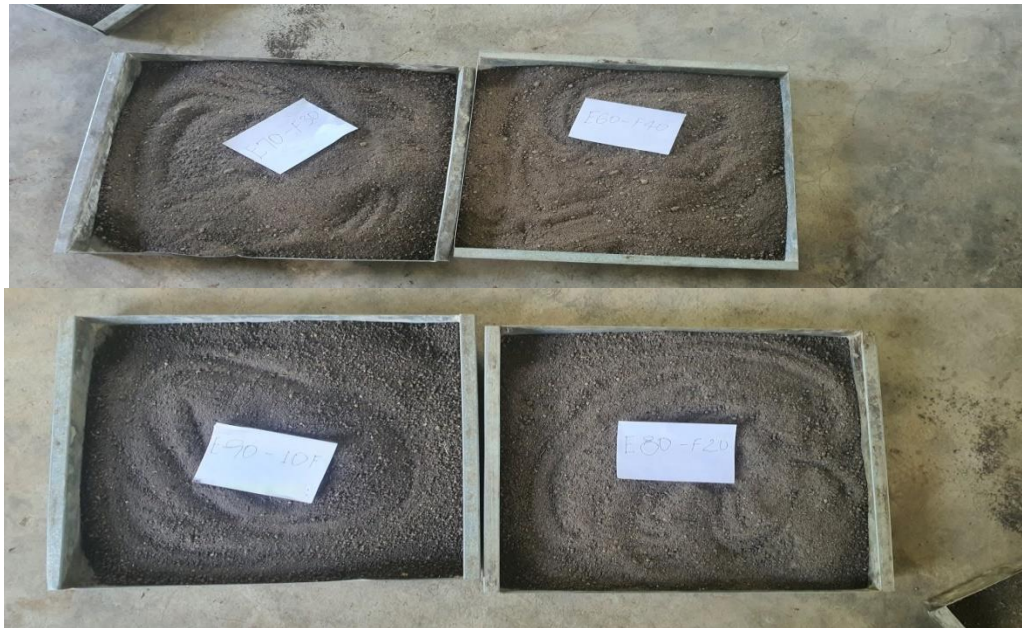
Figure 3. 3 Sample preparation with different percentage of soil-fly ash mix
