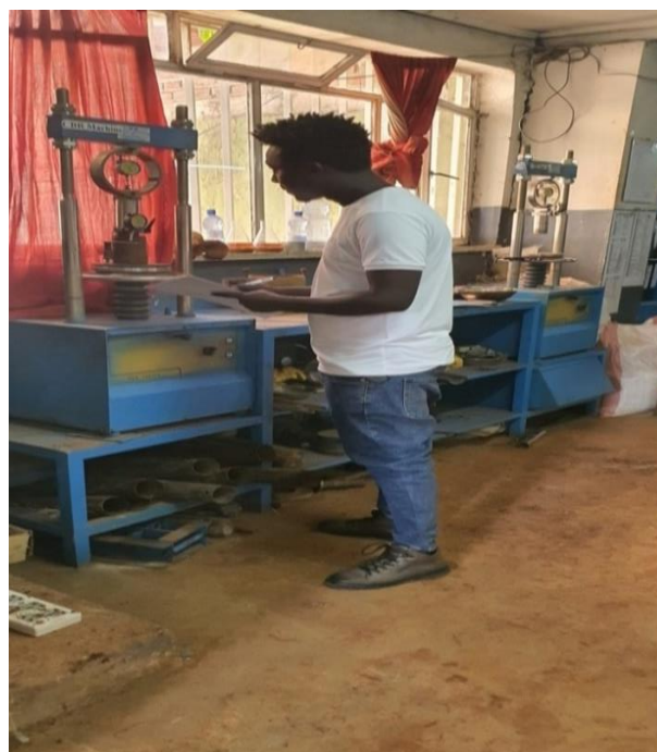
Figure D-12 UCS test reading
