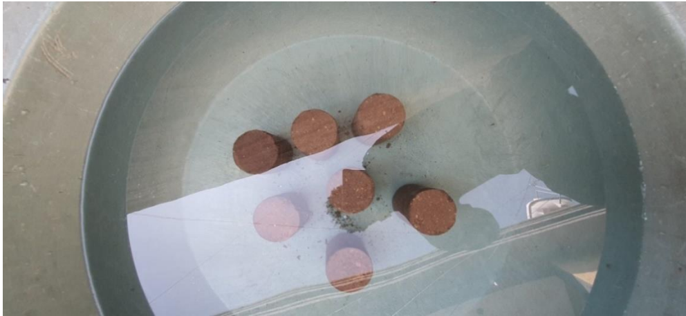
Figure 4. 20 Improved soil samples immersed in water for 48 h at 2nd cycle of wetting-drying
