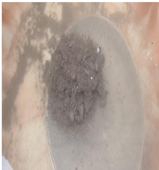
Figure 4. 18 Natural soil samples disintegrate before 48-hour immersion in water.
