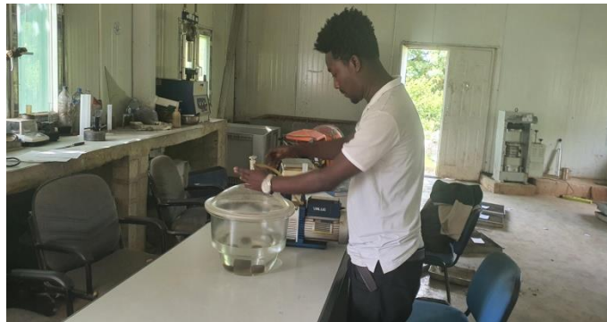
Figure D-13 Cyclic swelling saturation by using Vacuum pump
