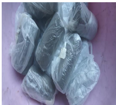
Figure D-16 UCS specimen preparation for curing
