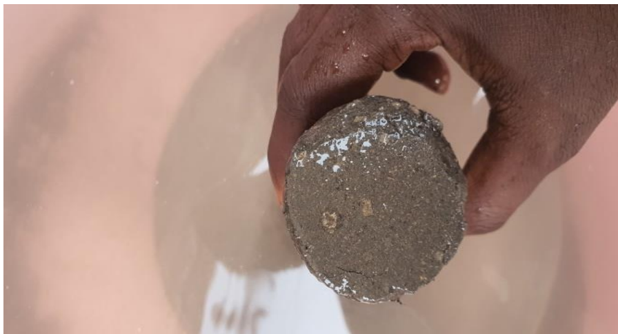
Figure 4. 22 Improved soil samples immersed in water for 48 h at 4th cycle of wetting-drying
