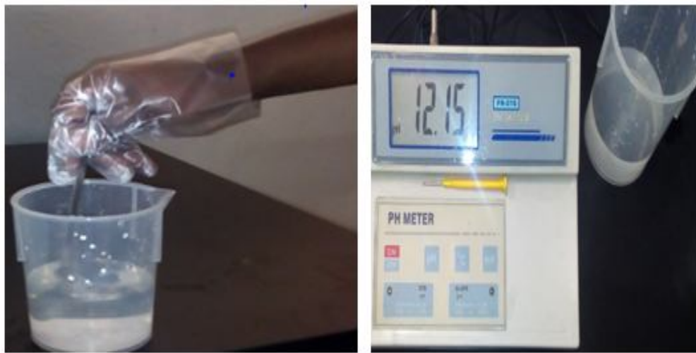
Figure 3.7 Mixing distilled water with Na OH and testing with ph meter
