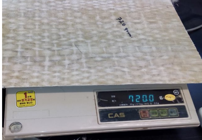
Figure 3.17: Measurement of specimen using digital balance.
