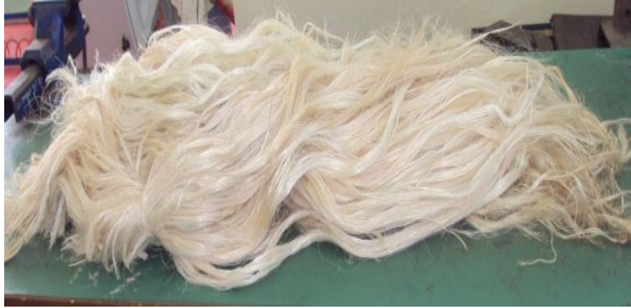
Figure 3.6 Extracted false banana fiber
