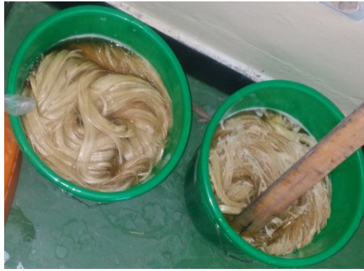
Figure 3.8 Soaking a fbf in base solution container for 24 hour.
