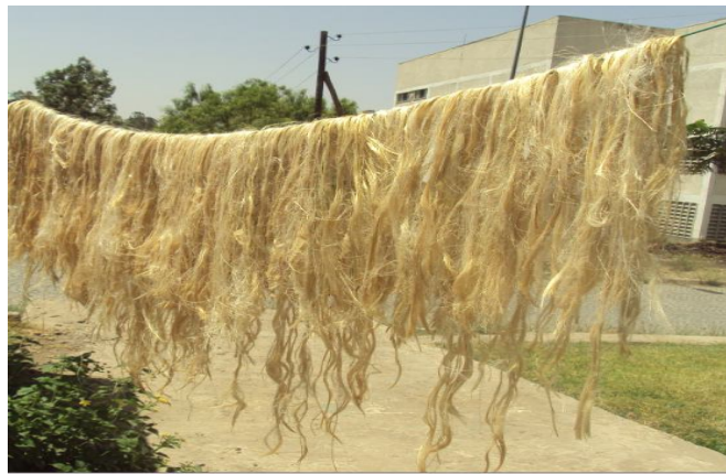
Figure 3.10 Exposing the false banana fiber to the sun light to dry.
