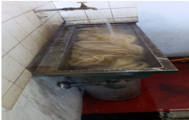
Figure 3.9 washing the soaked false banana fiber using tap water repeatedly.
