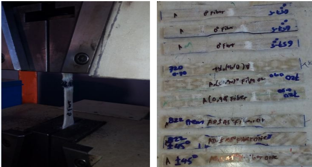
Figure 4.1: Specimen fractured by UTM tensile force.
