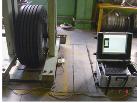
Figure 3.7: Testing retread tire deformation under vertical load
