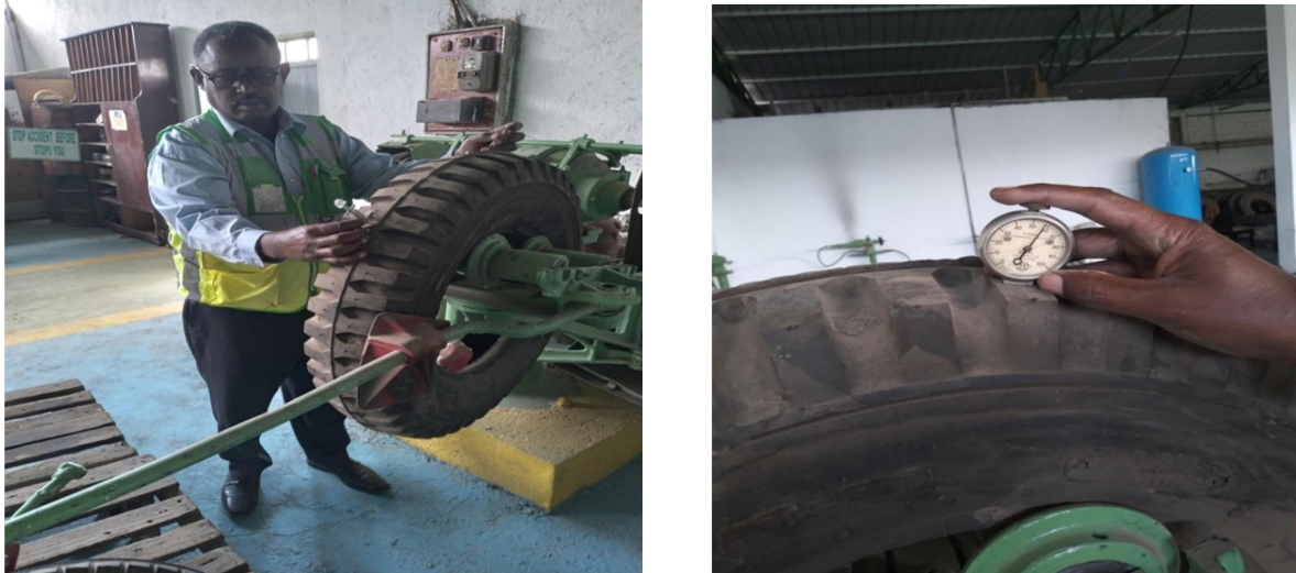
Figure 2.5: Final Inspection of hardness and tread depth
