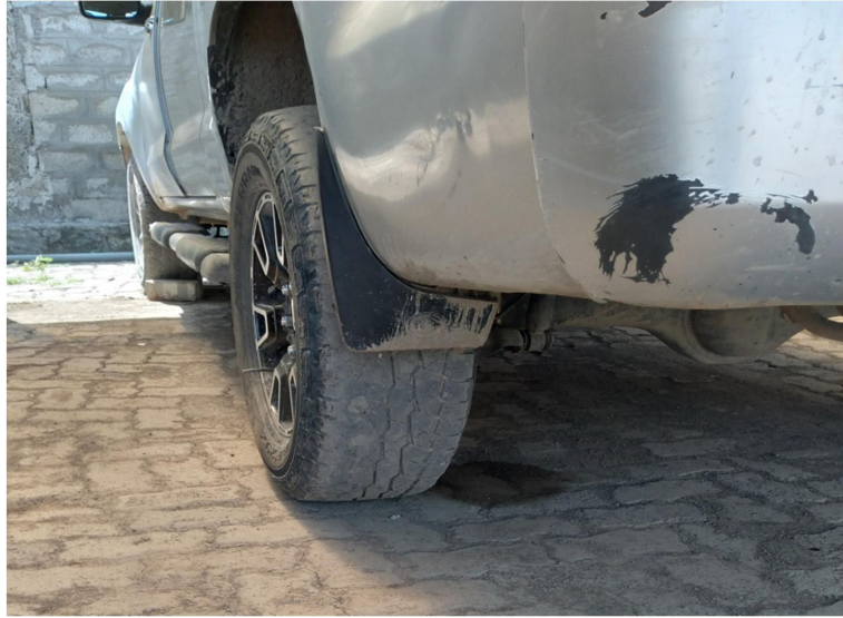
Figure 4.22: one of new tires removed from the study because of irregular wear
