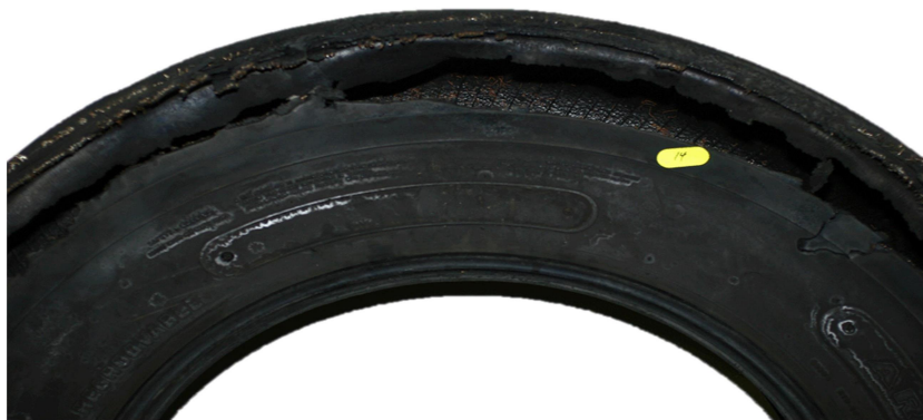
Figure 4.21: one of retread tires removed from the study because of tread separation
