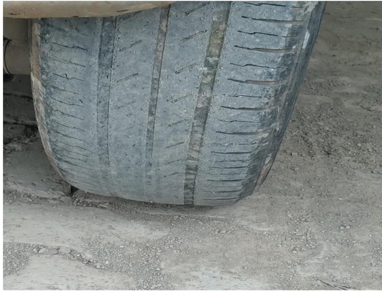
Figure 4.20: one of retread tires removed from the study because of excessive wear
