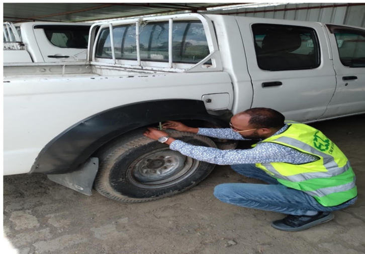
Figure 4.27: Measuring Tread depth
