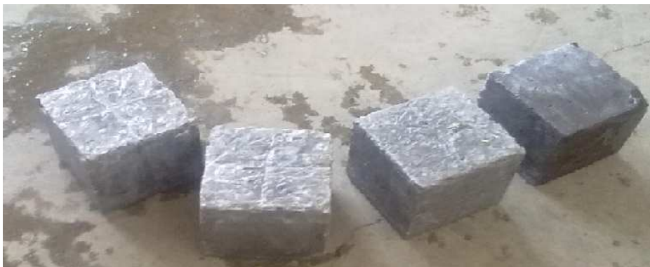
Fig.3.23Cubes ready for crushing
