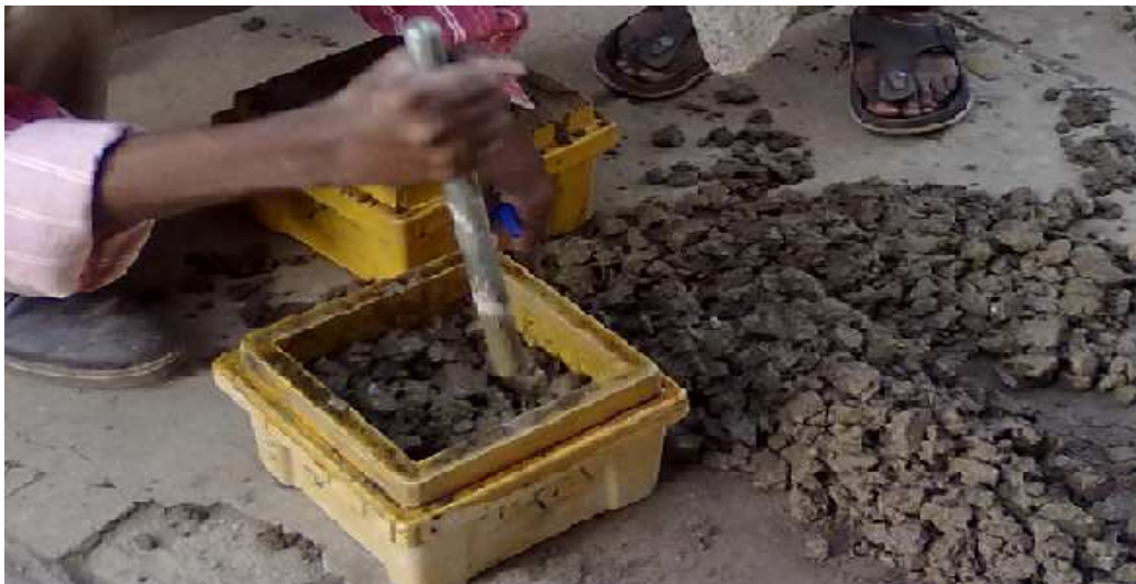
Fig.3.19. The cubes compacted in a layer
