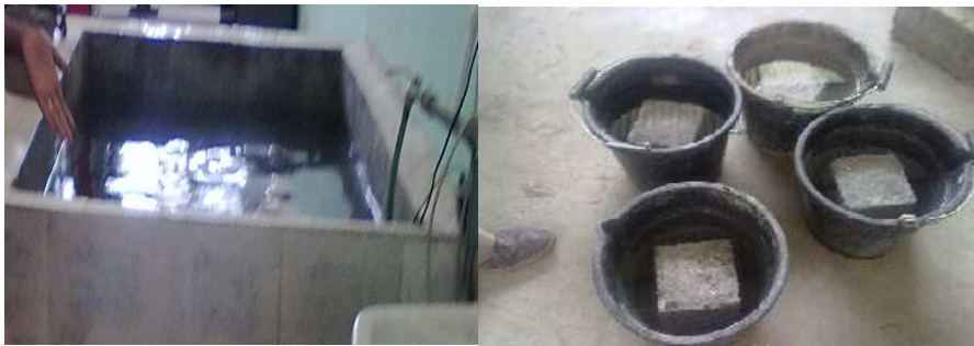
Fig.3.22. The cubes inter in to the curing tank
