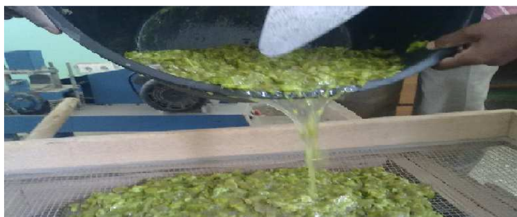
Fig.3.7.Separation of the gum by using sieves
