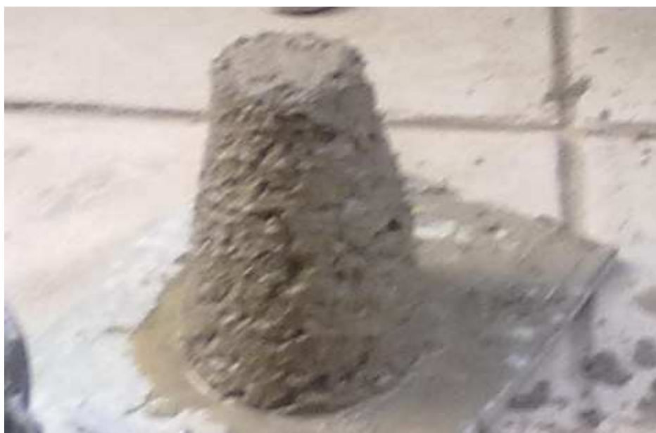
Fig.3.13. Shape of the slump with CG
