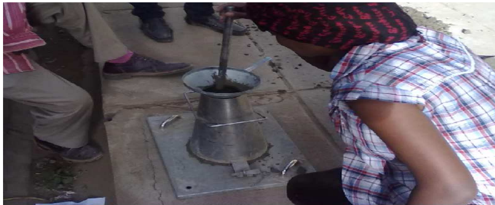
Fig.3.10.Rodding the concrete in three layers
