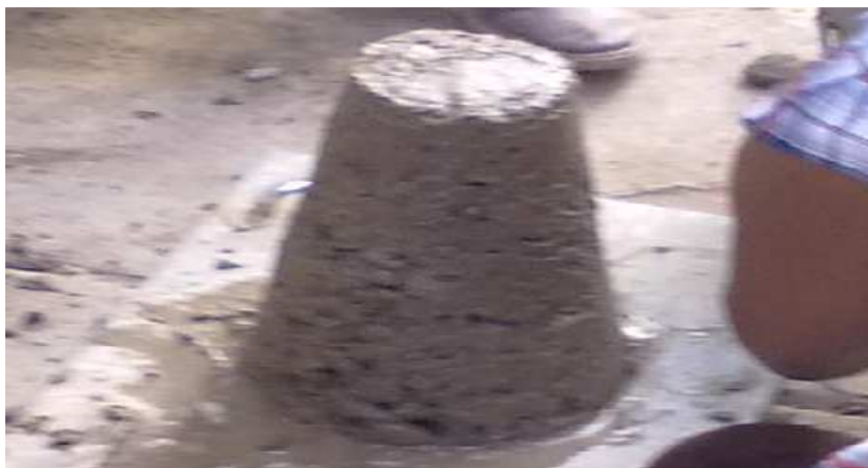
Fig.3.12. shape of the slump without gum
