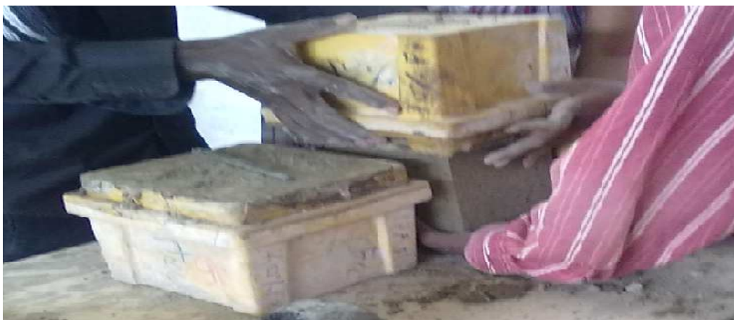
Fig.3.19. The cubes compacted in a layer
