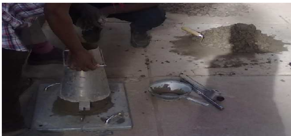
Fig.3.11. removing the slump cone without twisting
