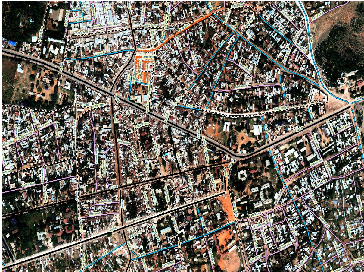
Figure 4.15: Geo-referenced digitized road network of Negelle City
