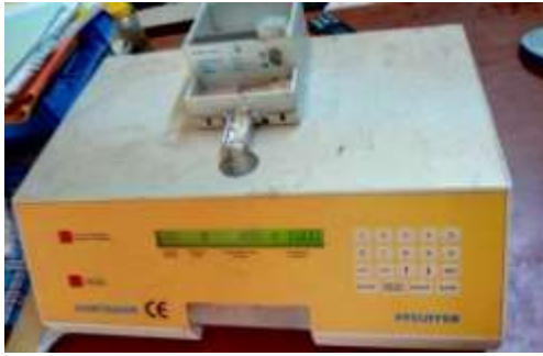
C, Seed-counter used to count threshed seeds
