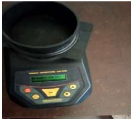
E, Electronic moisture meter
