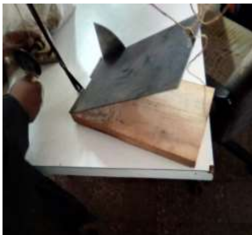
G, an instrument used to measure angle of repose as well as coefficient of friction.
