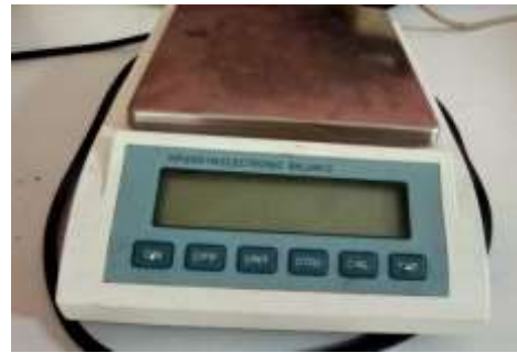
d, Electronic balances used to measure thousand grain mass
