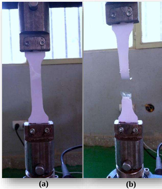
Figure 4. 3: PVC-sheet – before rupture (a), after rupture (b)
