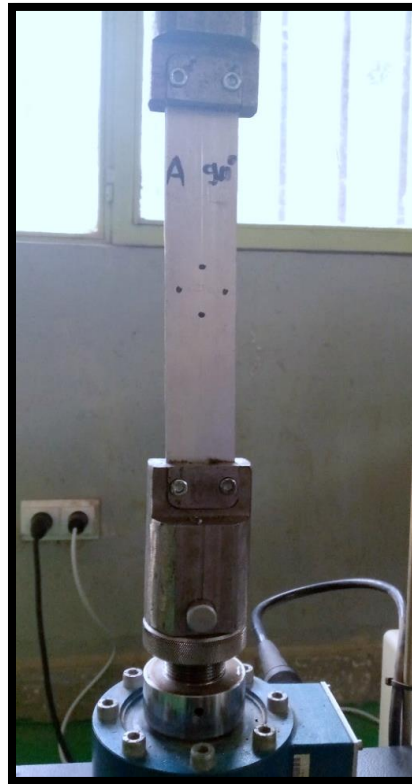
Figure 4. 10: Testing procedure – base material (Al-sheet)
