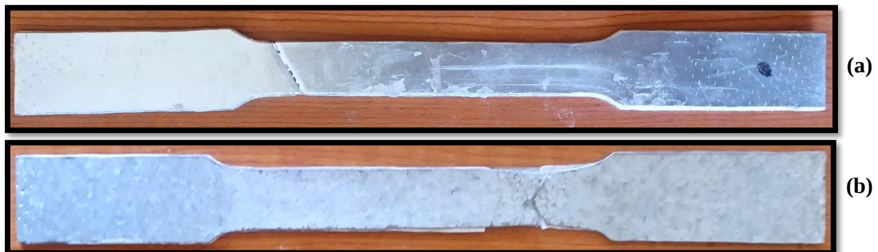
Figure 4. 5: MPM tensile tests – APA (a). GPG (b)– after rupture
