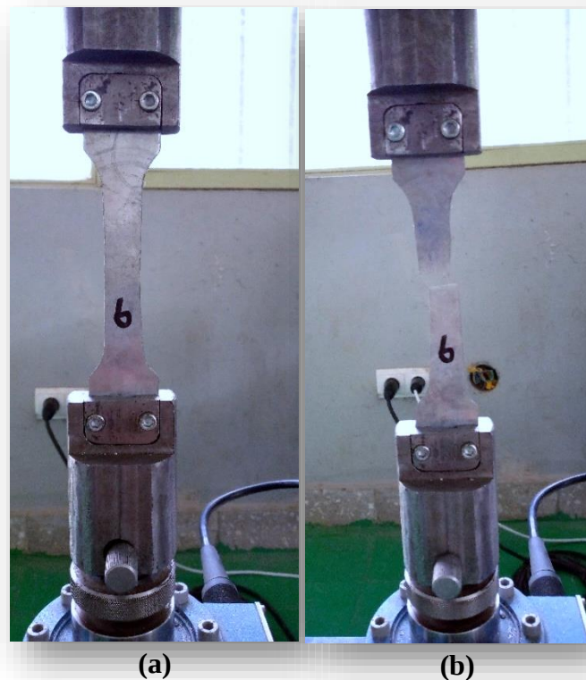
Figure 4. 1: GSS tensile test ( 90^\circ orientation) – before rupture (a), after rupture (b)
