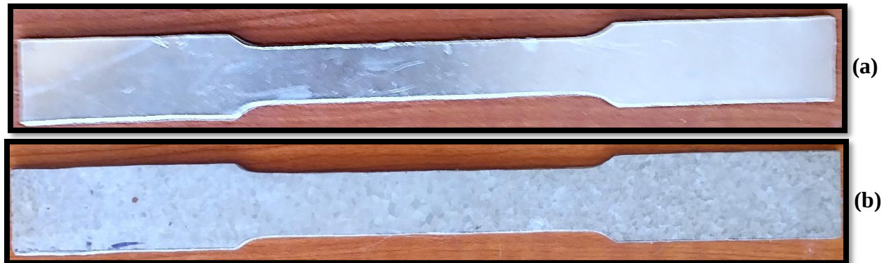
Figure 4. 4: Tensile test specimens – APA (a), GPG (b)– before deformation
