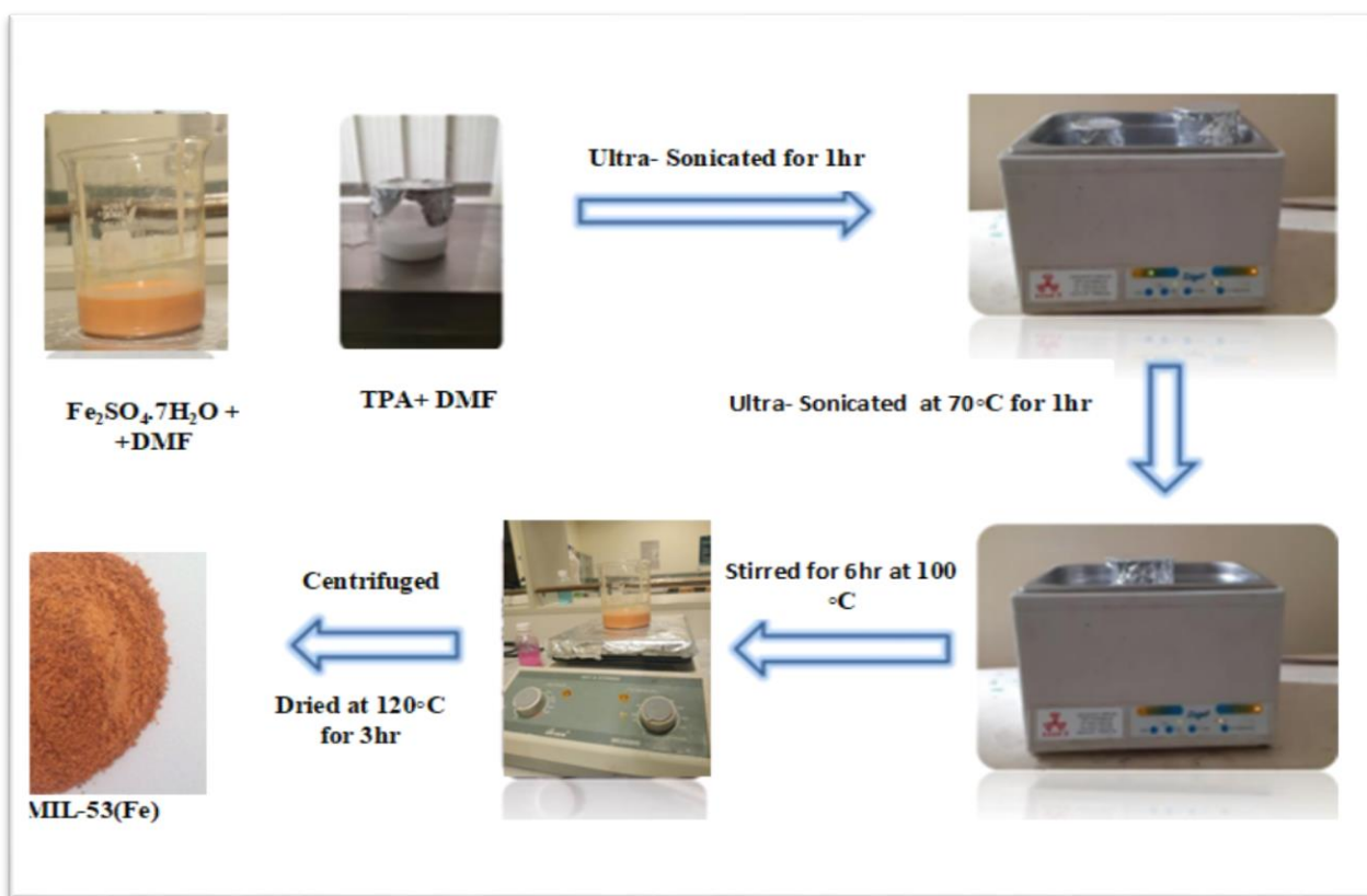
Figure 3. 2: Schematic illustration of the MIL-53(Fe) formation process.
