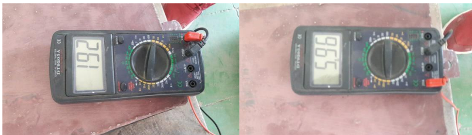
Figure 20: Input voltage and current measurement
