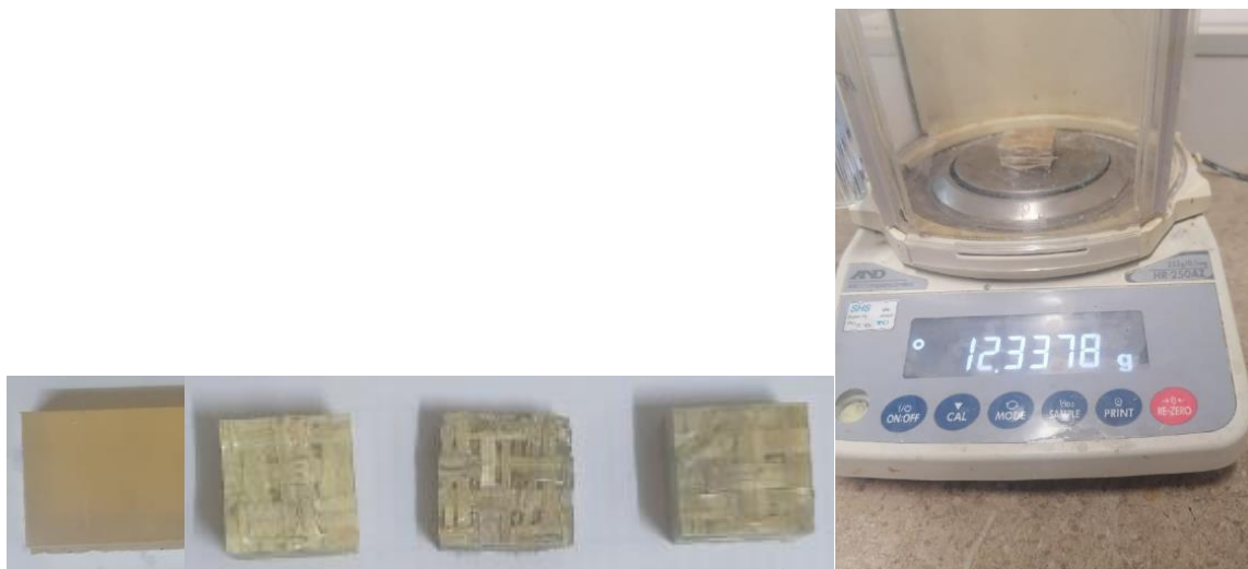
Figure 3.21: Specimens and measuring specimen mass using weight balance.
