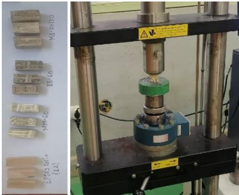
Figure 3.18: Compression specimens and testing setup.
