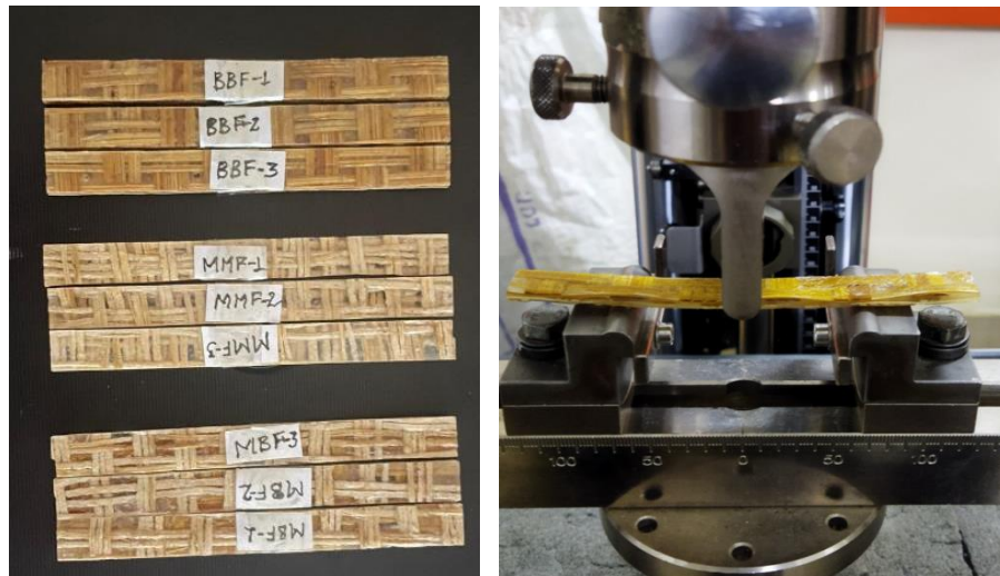
Figure 3.17: Bending specimen and its testing setup.
