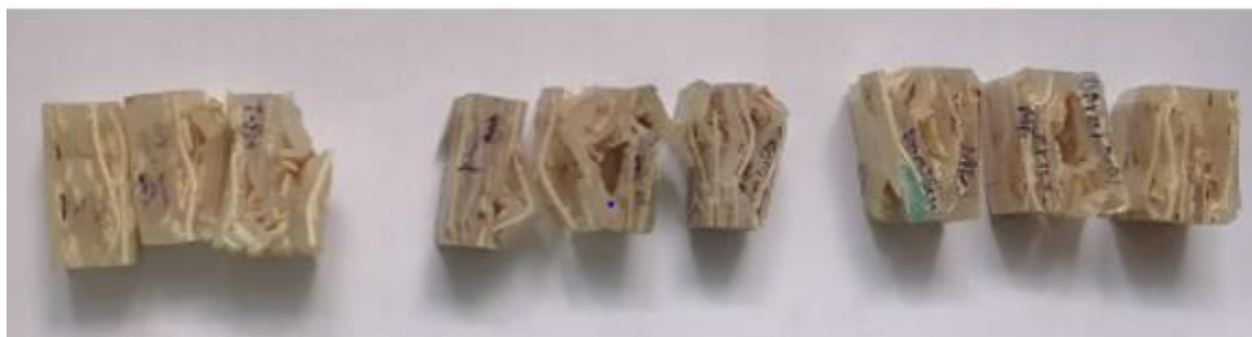
Figure D.1. Compressive specimens after testing.
