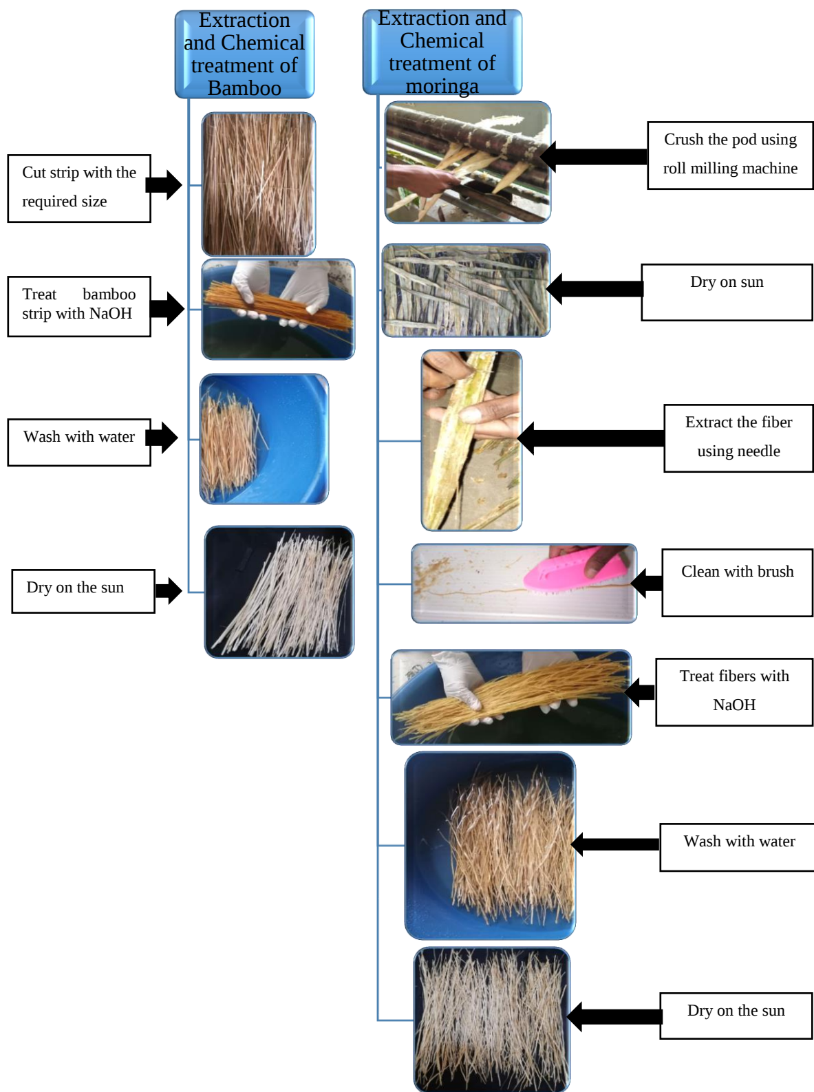
Figure 3.6: Pictorial summary of extraction and chemical treatment of moringa and bamboo fibers.
