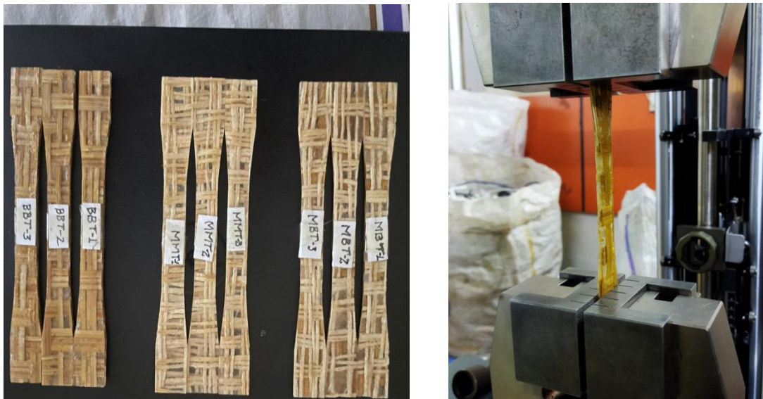
Figure 3.16: Tensile test specimens and testing setup.
