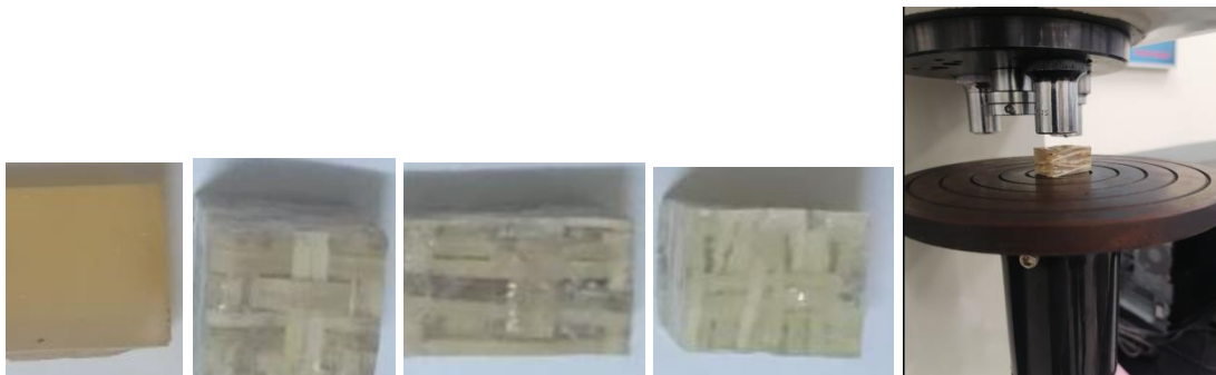
Figure 3.20: Hardness specimens and Vickers Hardness Tester
