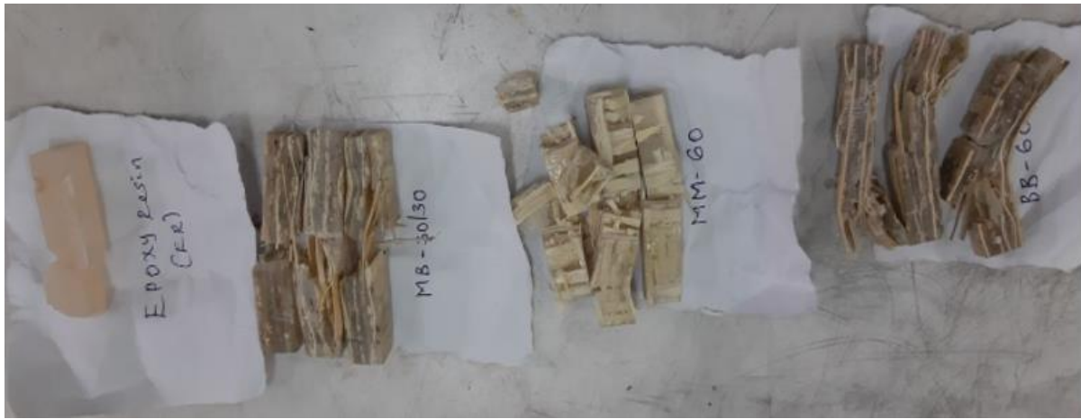
Figure D.2. Impact specimens after testing.
