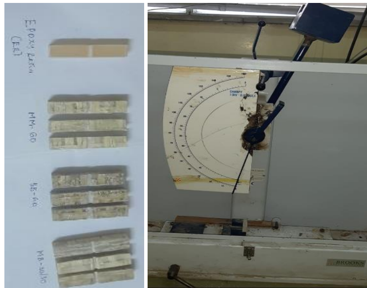
Figure 3.19: Impact specimens and testing machine.
