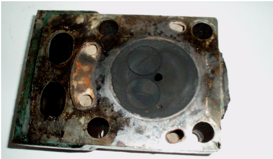
Figure 4.7 Carbon deposits on cylinder head with cotton seed oil blended fueled engine operation
