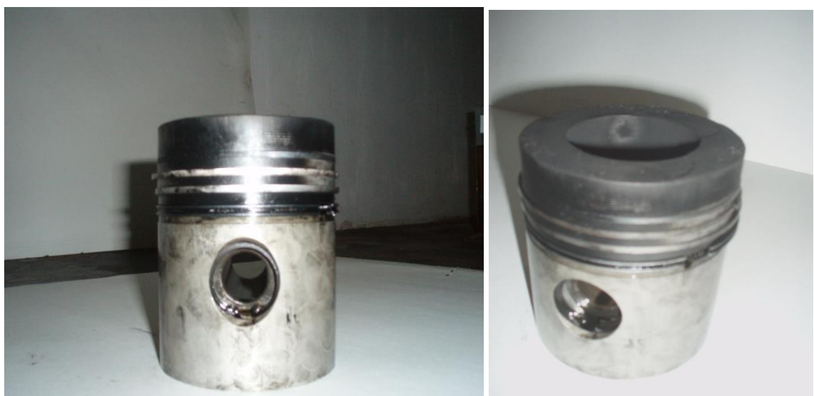
Figure 4.5 Piston top surface and ring sticking with diesel fueled engine and cotton seed blended oil fueled engine operation.
