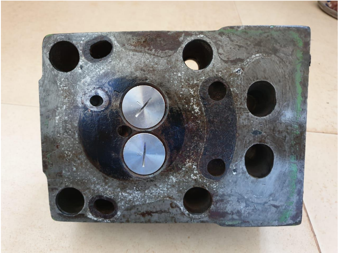
Figure 4.6 Carbon deposits on cylinder head with diesel fueled engine operation with new valves
