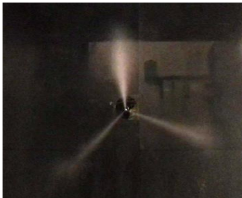
Figure 3.9 Injector spray from orifice
