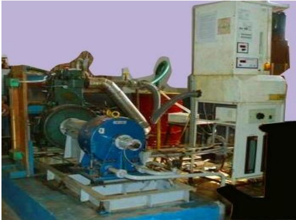
Figure 3.8 single cylinder four stroke DI compression ignition engine test rig.
