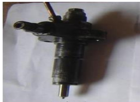
Fig 3.10 Injectors containing 3 Hole
