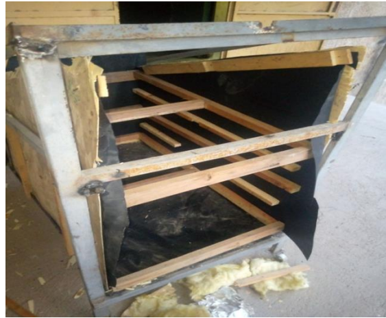
Figure 3.11 Construction of drying chamber
