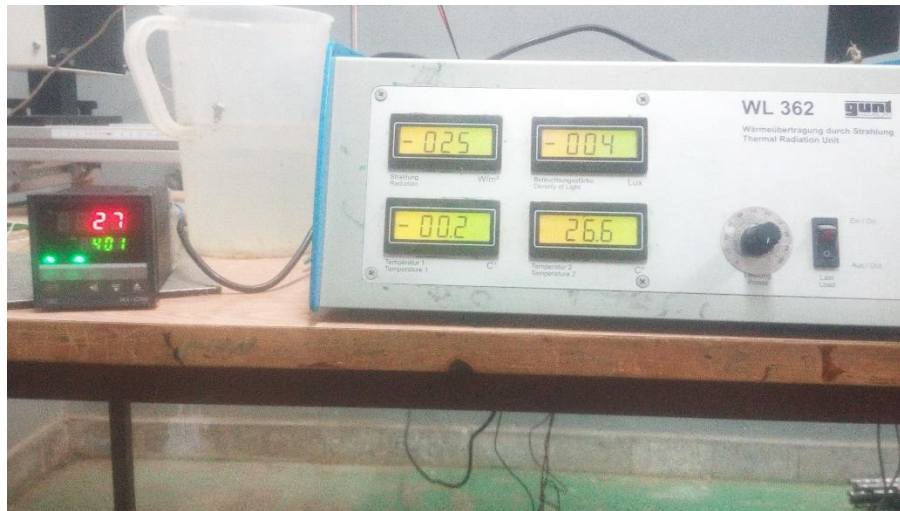
Figure A.1 Calibration of single thermocouple with laboratory standard thermopile
