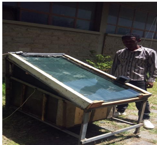
Figure 3.12 Solar kiln experimental setup unit
