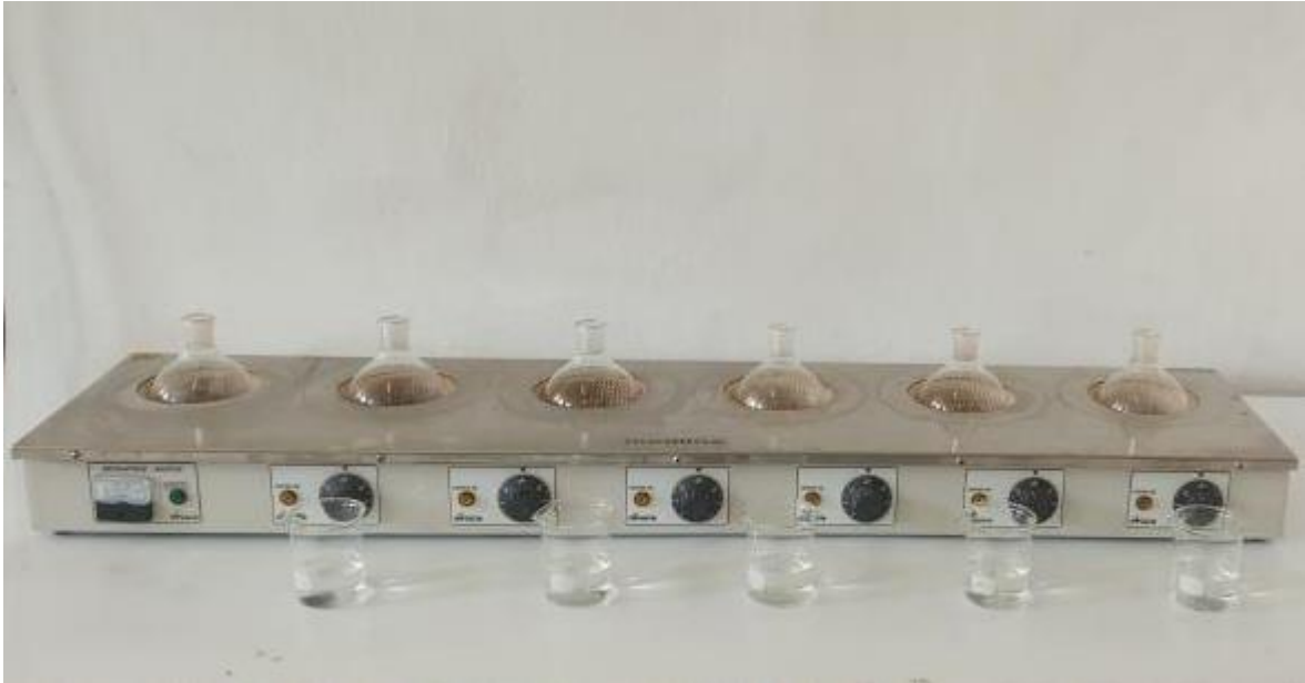
Figure 3.3: Experimental set up of caustic treatment
