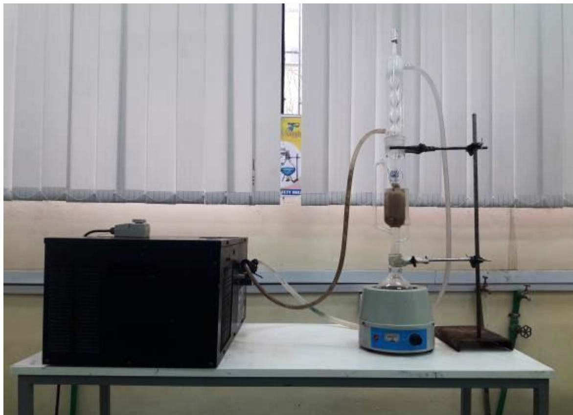
Figure 3.2: Experimental set up of Soxhlet solvent extraction
