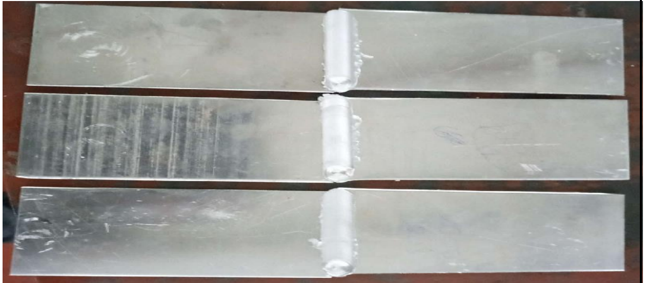
Figure 4.3 welded sample of aluminum alloy 6023 T6 at different parameters
