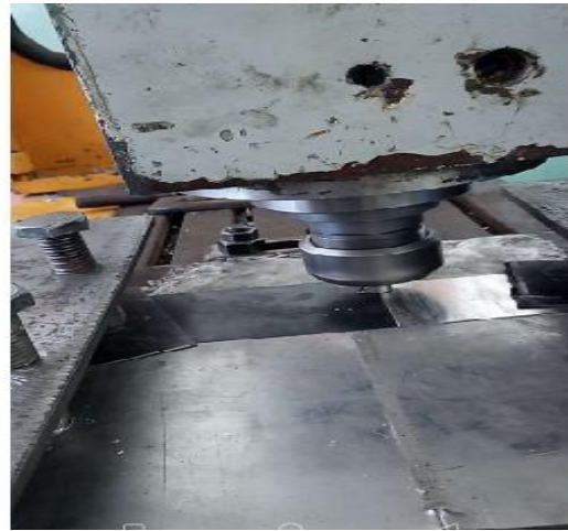
b) Backing plate secured on milling machine during FSW
