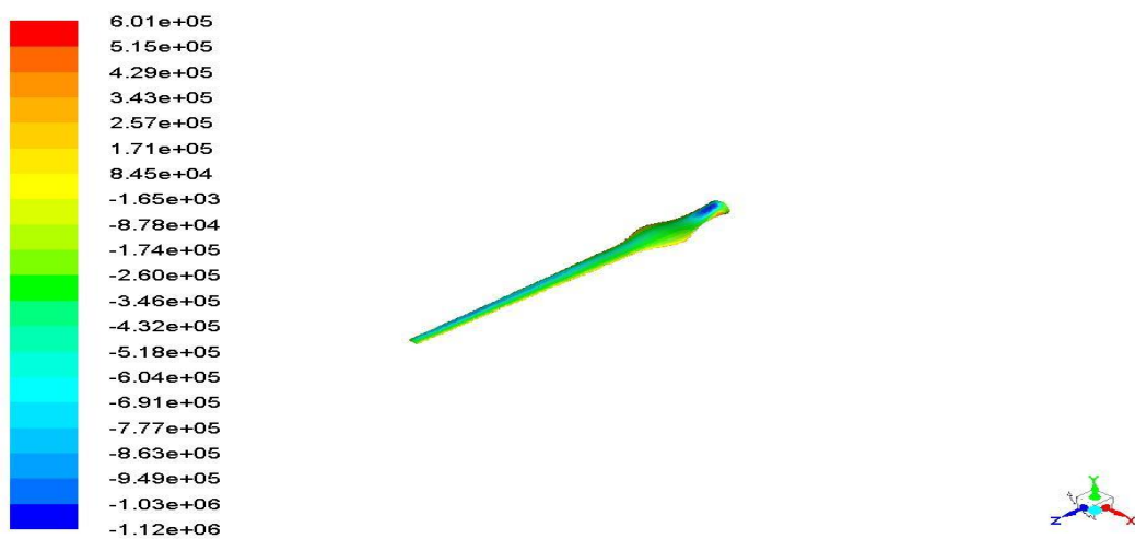
Figure 6.12 : Suction Side Pressure Contour At \alpha = 5^\circ
