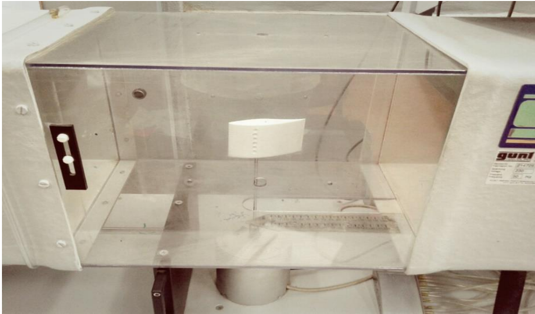
Figure 5.7 : Dimpled S830 Model on Test Section
