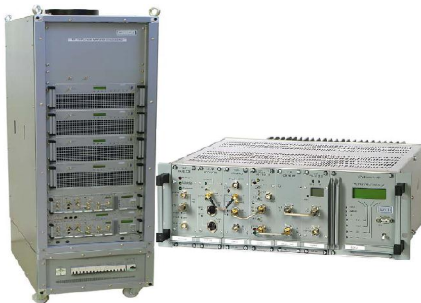
Fig.3.4. Air cooled VHF B-III ORTVO station transmitter
