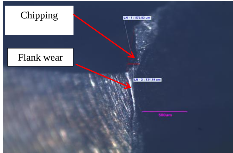
Figure 4-10: Optical microscope micrograph of drill bit wear of 10mm diameter
