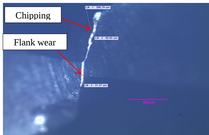
Figure 4-9: Optical microscopic image of drill bit tip wear of 8mm diameter
