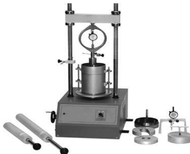
Figure 2: CALIFORNIA BEARING RATIO (CBR) TEST APPARATUS (NICOLAIDES, 2014)
