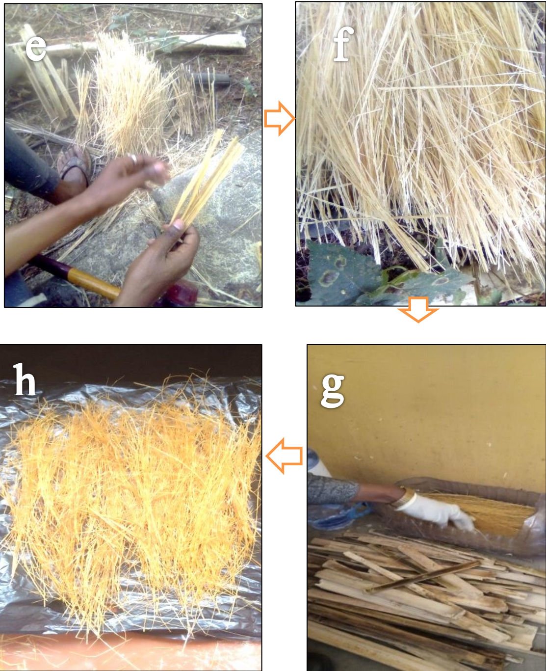
Figure 3.2. Bamboo fiber extraction technique (a) bamboo plant (b) dry bamboo plant, (c) split bamboo clam, (d) the cleaved bamboo strips are soaked under the water in the bath (e) wetted bamboo strips are hammered with a rubber hammer (f) illustrates the outcome of the extracted bamboo fiber (g) alkaline treatment (h) treated bamboo fiber.
