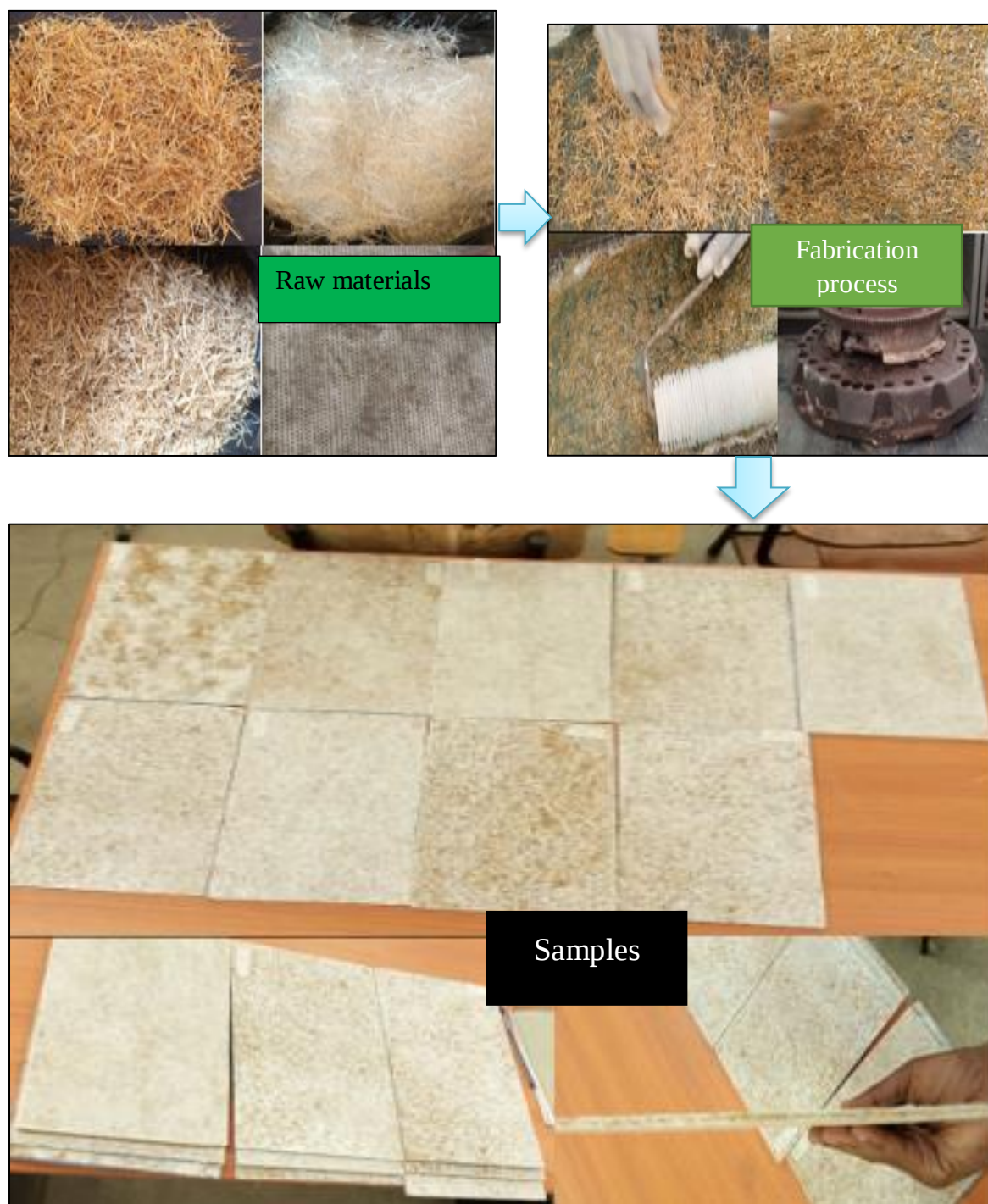
Figure3.8. Composites samples fabrication process.
