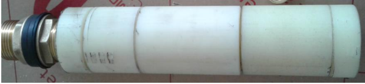
Fig.3.1: venturi tube: (a) drawing of venturi tube and (b) manufactured venturi tube.
