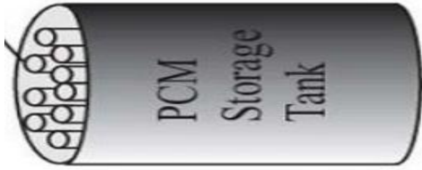
Figure 5. 7. Schematic configuration of shell and tube latent heat thermal energy storage system (LHTES) unit with a complete system, and concentric cylinders (Tehrani et al., 2016).
