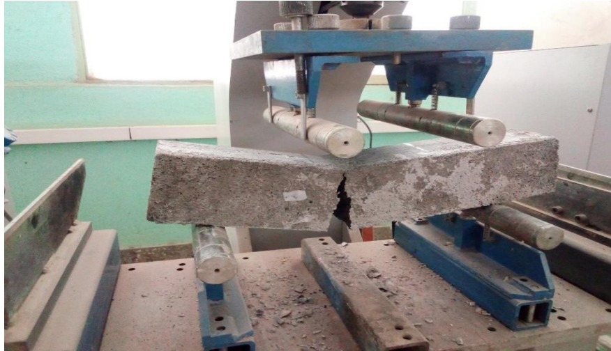
Figure 3. 6. Flexural Sample Testing
