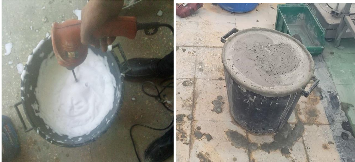
Figure 3. 5.Generated foam using hand driller machine
