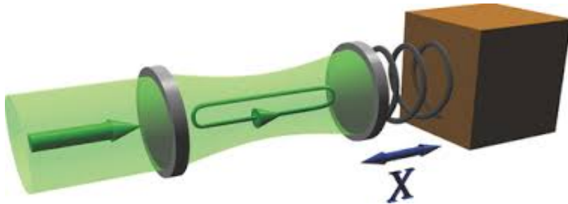
Figure 1: A cavity optomechanical system consisting of a Fabry Perot cavity with a harmonically bound end mirror
