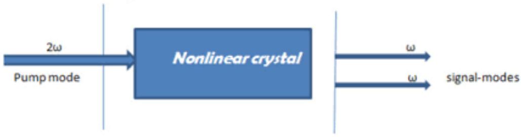
Figure 3: A degenerate parametric amplifier with nonlinear crystal pumped by coherent light.
