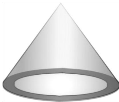
Figure 2.1 Hollow cone spray pattern [Shull, 2012]
