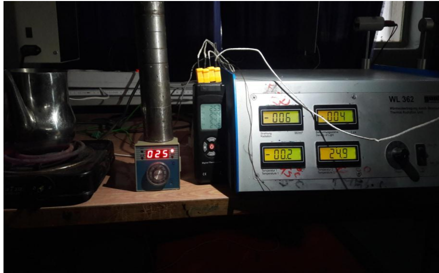
Figure 12. temperature readings of the measuring device (thermometer) and the other two digital thermometers during calibrations.
