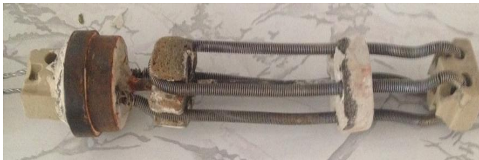
Figure 13. The Electrical heater
