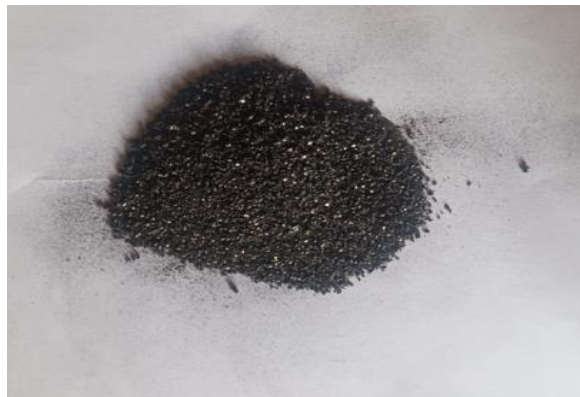
Figure 4.35 chip formed during machining of flake graphite cast iron.
