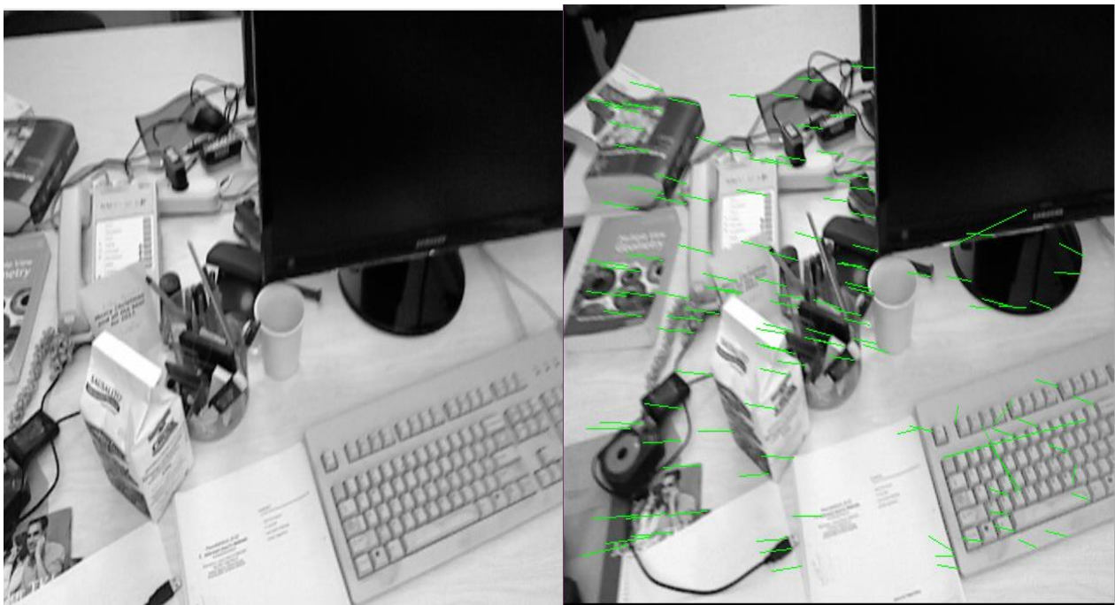
Figure6. 4 extraction using minutiae points (Key points) from consecutive frames
