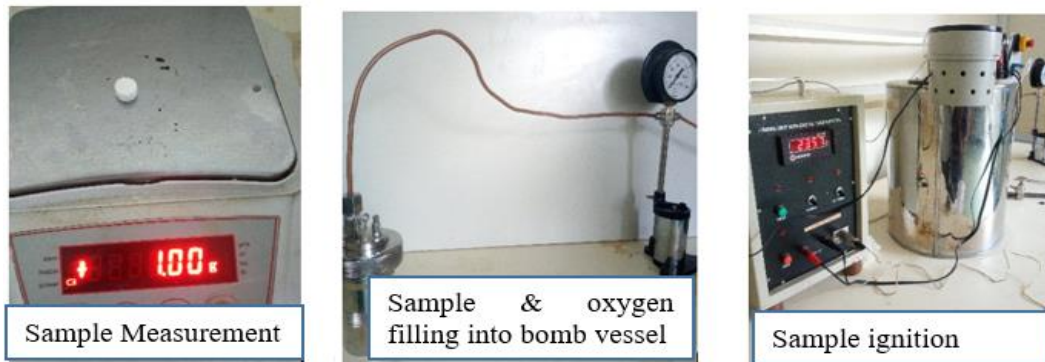
Figure 3.4 Measuring Samples Calorific Value
