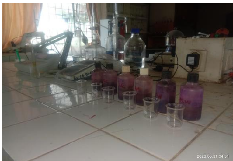
Figure 5. Compost /Feedstock sample preparation for PH and EC analysis ,Ethiopian sugar industry group research laboratory
