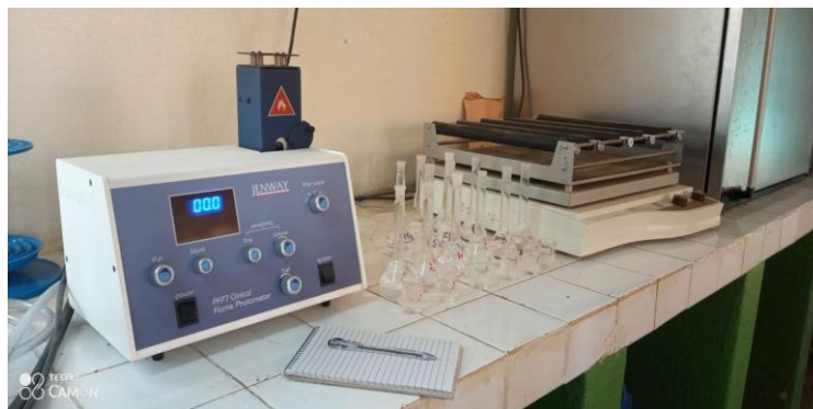
Figure 8. Flame photometer and prepared samples for Potassium analysis, Ethiopian sugar industry group research laboratory
