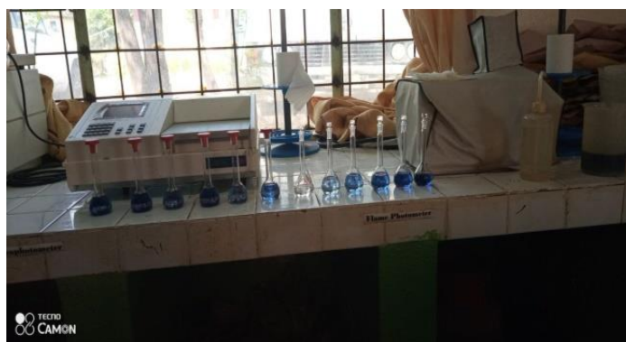
Figure 7. Spectrophotometer and prepared samples for phosphorus analysis, Ethiopian sugar industry group research laboratory
