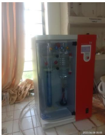
Figure 6. Kjeldahl auto distillation unit on nitrogen analysis, Ethiopian sugar industry group research laboratory
