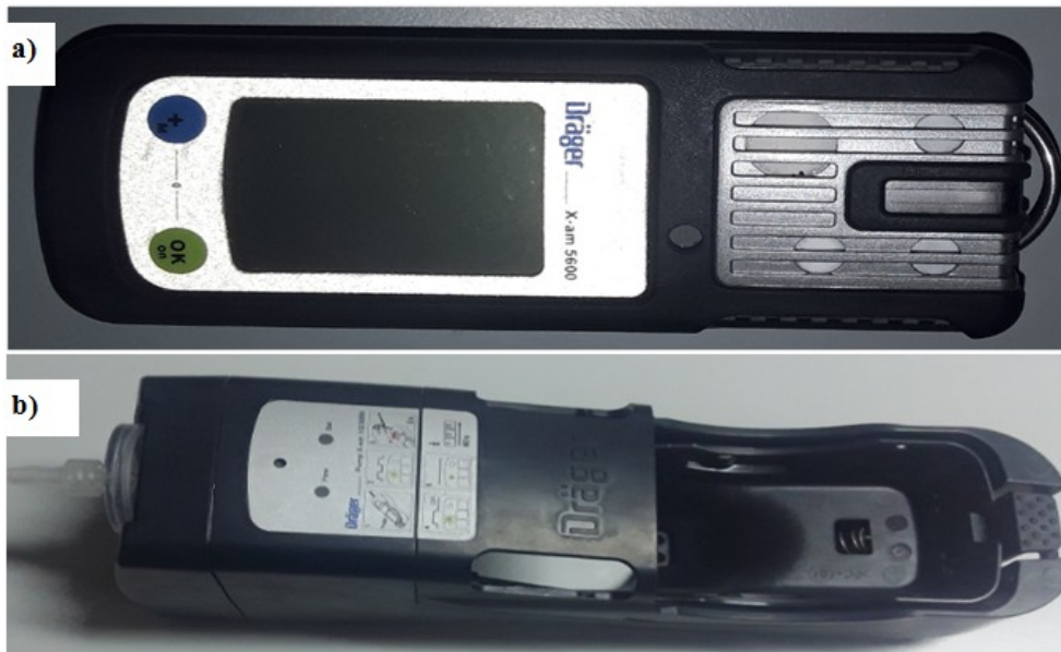
Figure 2: Multi Gas Detection Device a) X-am-5600 b) Calibration cradle
