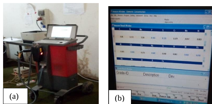
Figure 3.10 Spectrometer (a) machine tool, (b) result display window
