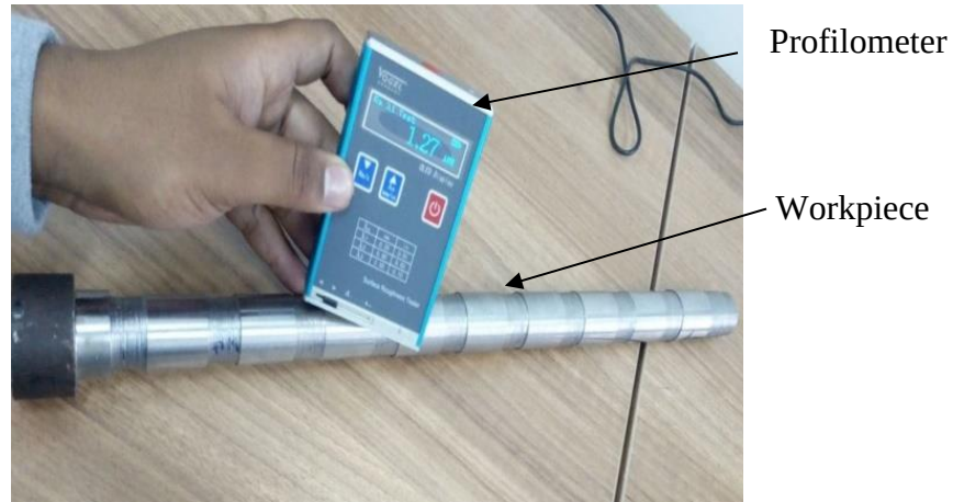
Figure 3.14 Surface roughness testing by using a surface contact profilometer
