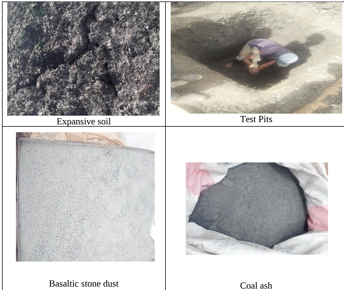
Figure 3. 2 Photographic view of expansive clay soil, stone dust and coal ash used in present study
