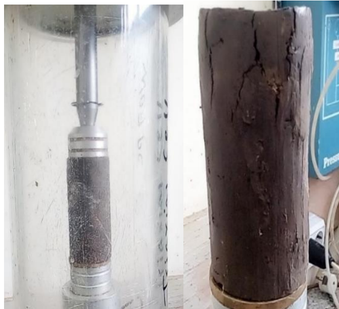
Figure 3. 8 The photographic view of Unconfined compressive strength test
