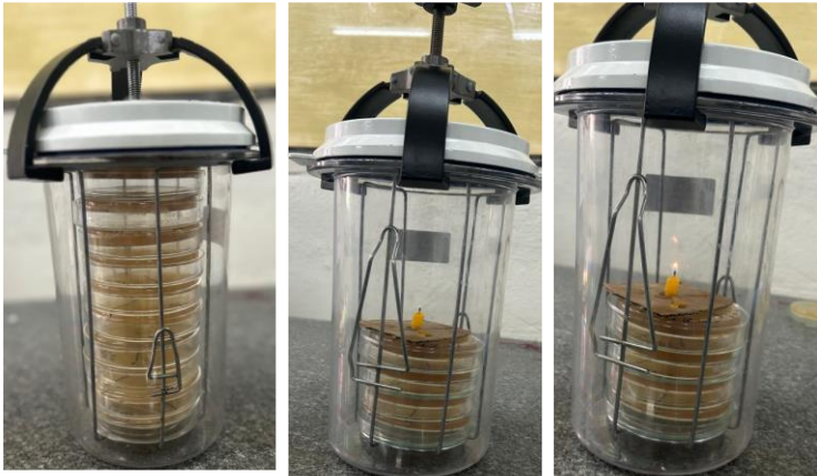
Figure -A 2 : An anaerobic jar is an instrument used in the production of an aerobic environment. This method of anaerobiosis, as others is used to culture bacteria that die or fail to grow in the presence of oxygen (anaerobes).
