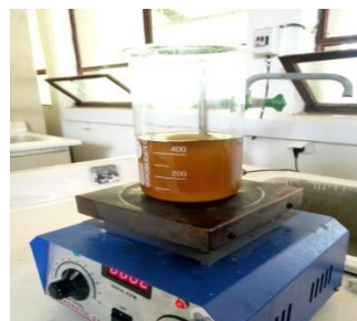
Fig.3.5 Transesterification of Jatropha and Castor oil
