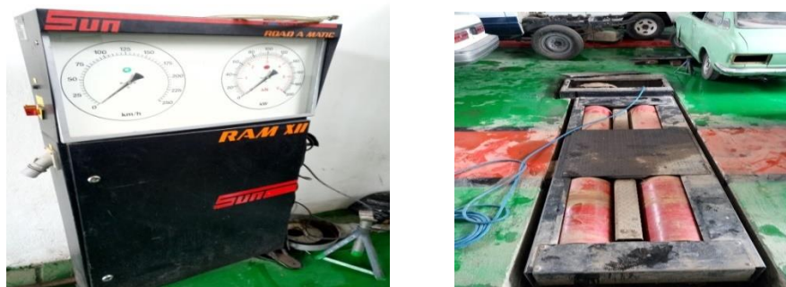
Fig. 3.11 Sun ROAD-A-MATIC RAM XII Chassis Dynamometer
