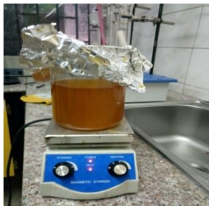
Fig.3.5 Transesterification of Jatropha and Castor oil
