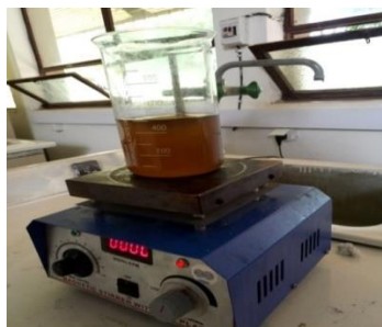
Fig.3.4 Preheating of the oil
