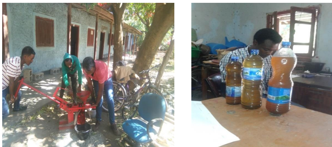
Fig.3.2 Mechanical pressing of Jatropha seed.
