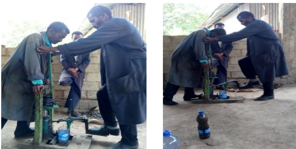
Fig.3.3 Mechanical pressing of Castor seed
