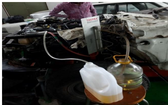
Figure 3.13 Fuel consumption measurement setup
