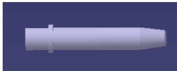
Figure 3.4. CATIA model of plunger.
