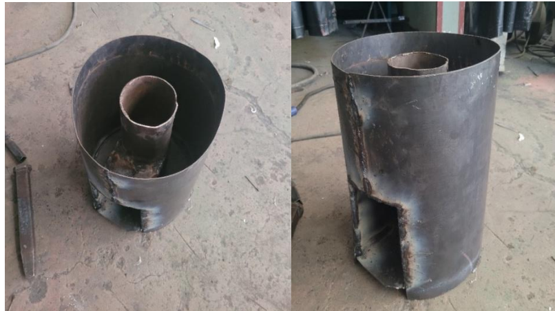
Figure 4.2 Combustion chamber and body of the rocket stove
