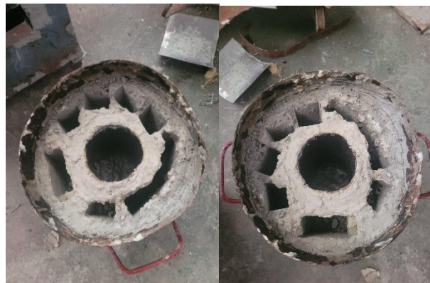
Insulation material pouring into the shapes
