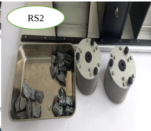
Fig3.18 Slake durability test for RS2
