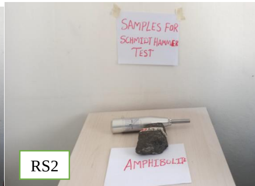
Fig3.4 schimdt Hammer Test for RS2
