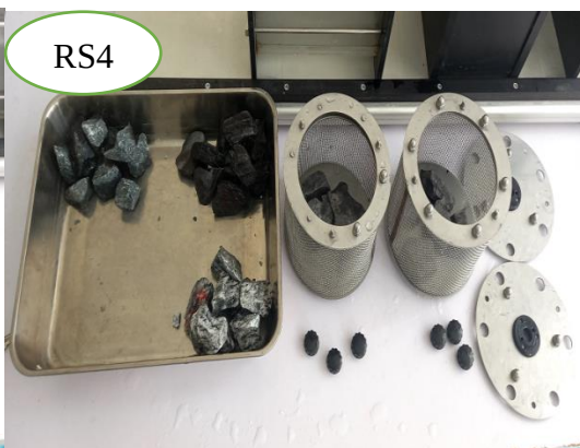
Fig3.20 Slake durability test for RS4
