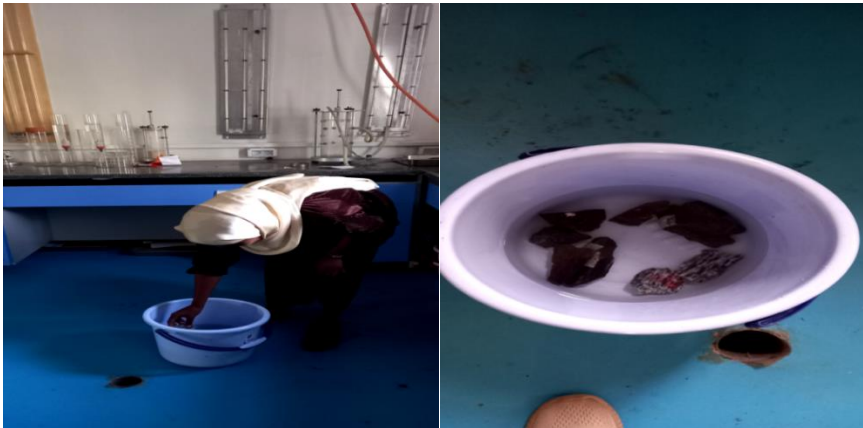
Fig3.13 Conducting Saturated density test for rock samples
