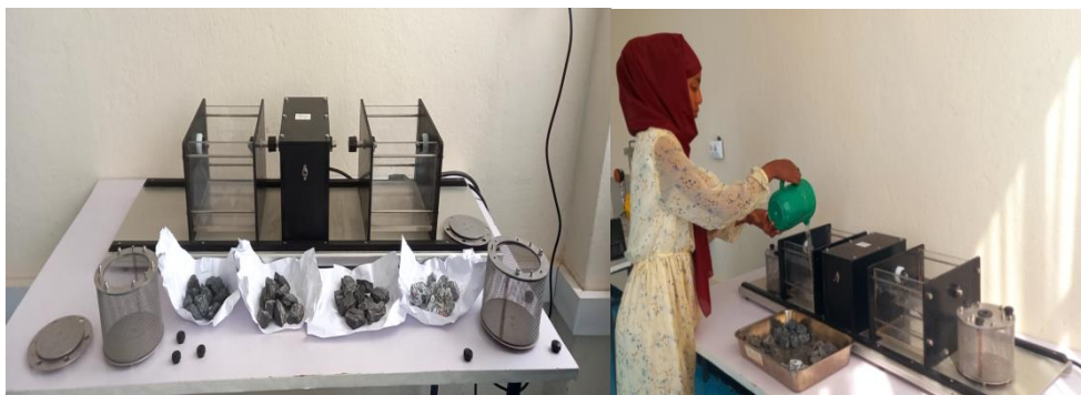
Fig3.16 Conducting slake durability test
