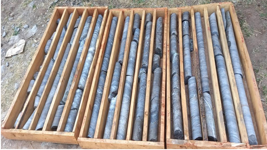
Fig3.21 Core drilling data from Sakaro underground tunnel
