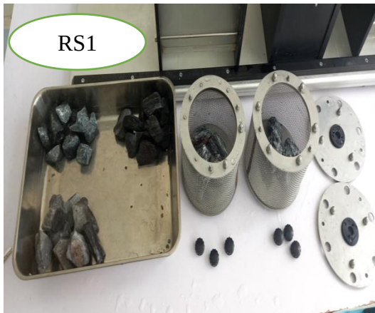
Fig3.17 Slake durability test for RS1
