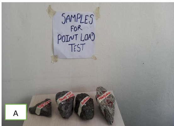
Fig 3.8 A) Rock samples before Conducting point load test
