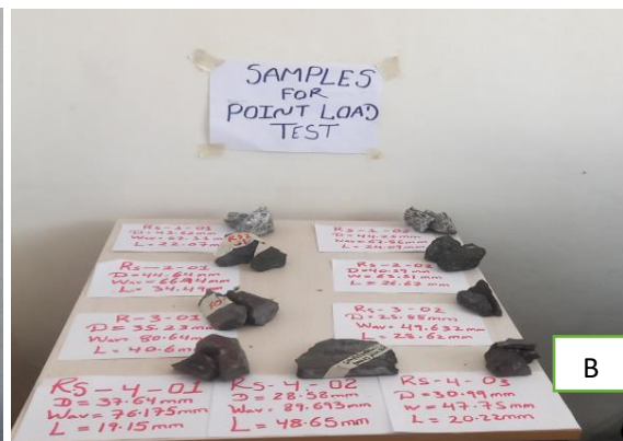
Fig3.9 B) Rock samples after Point load test is done
