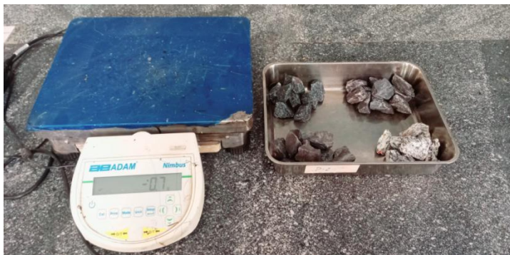
Fig3.15 Preparing rock samples for slake durability test
