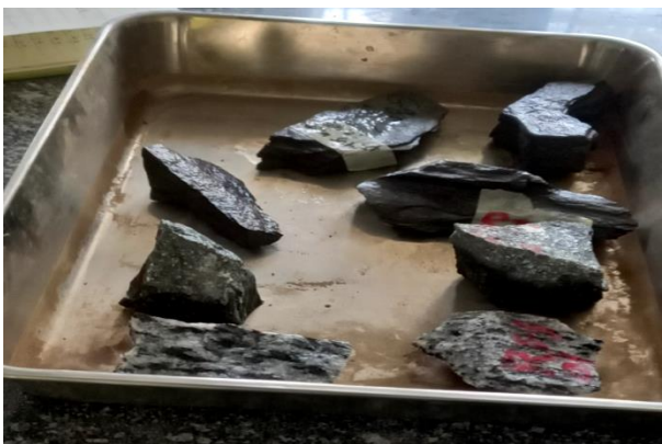
Fig3.14 Rock samples obtained from saturated density test after being placed in water for 24 hours
