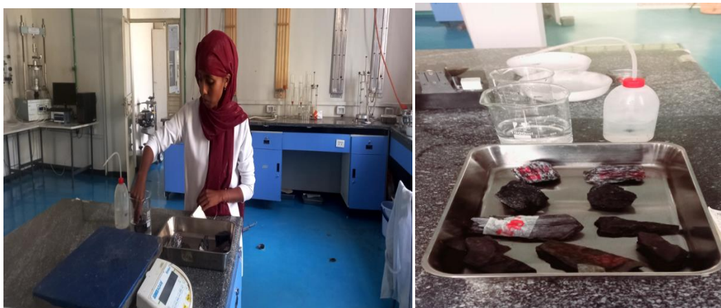
Fig 3.11 Measuring the volume of rock samples and preparing them to be oven dried for 24 hours
