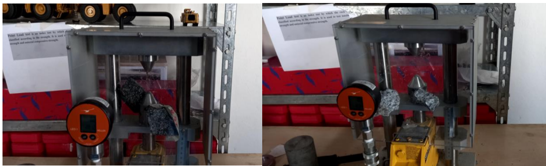
Fig3.7 Point load test of rock samples
