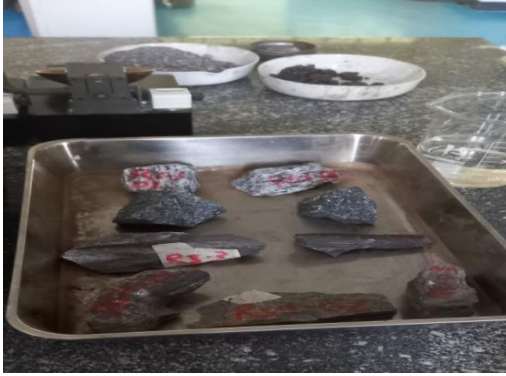
Fig3.12 preparing rock samples to conduct saturated density test
