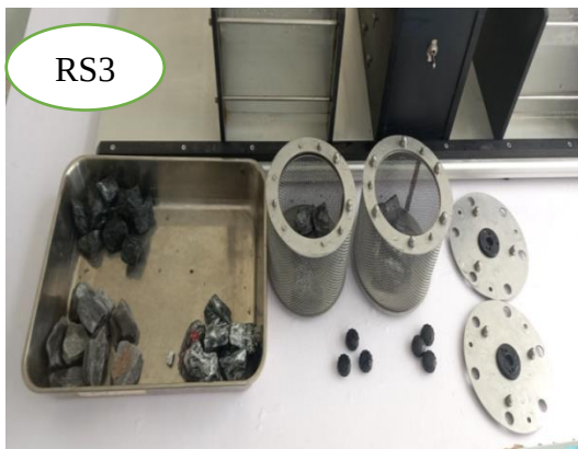
Fig3.19 Slake durability test for RS3
