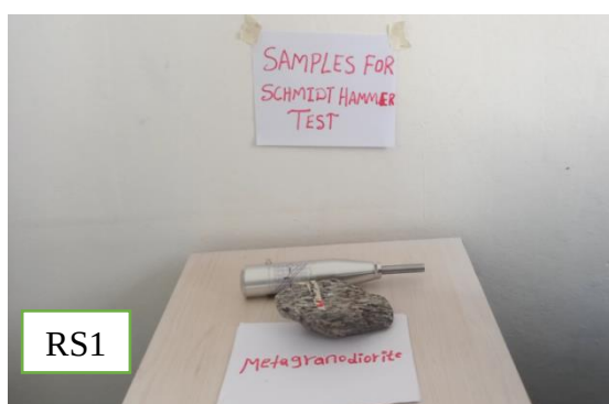
Fig3.3 schimdt Hammer Test for RS1
