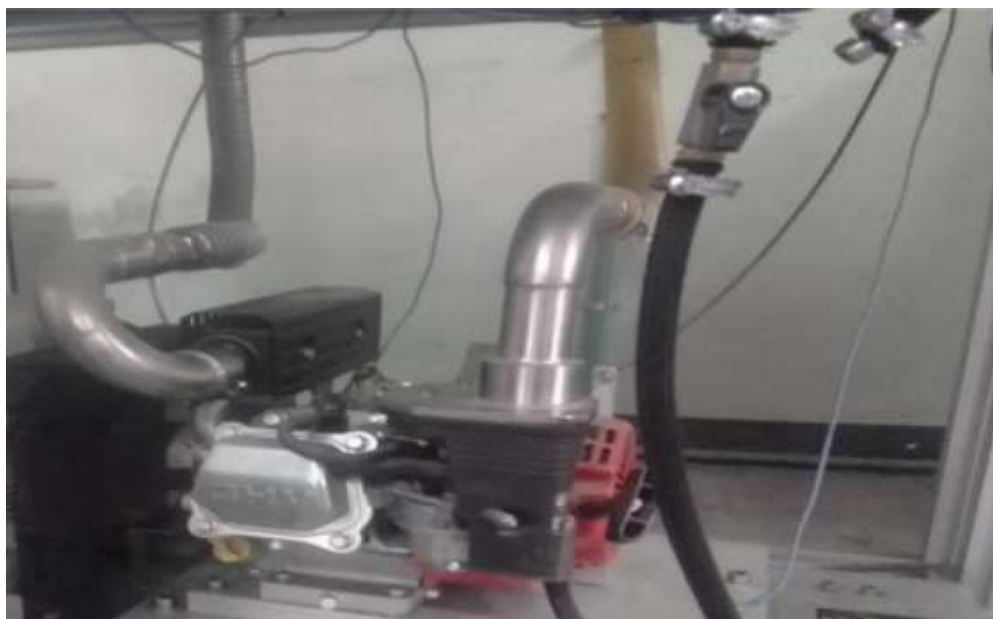
Figure: 3.3 TBMC3-01 Engine used for the test
