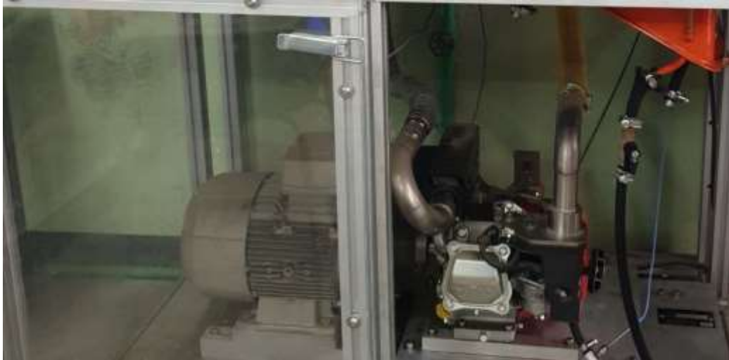
Figure. 3.8 Engine connected with dynamometer for the test set up
