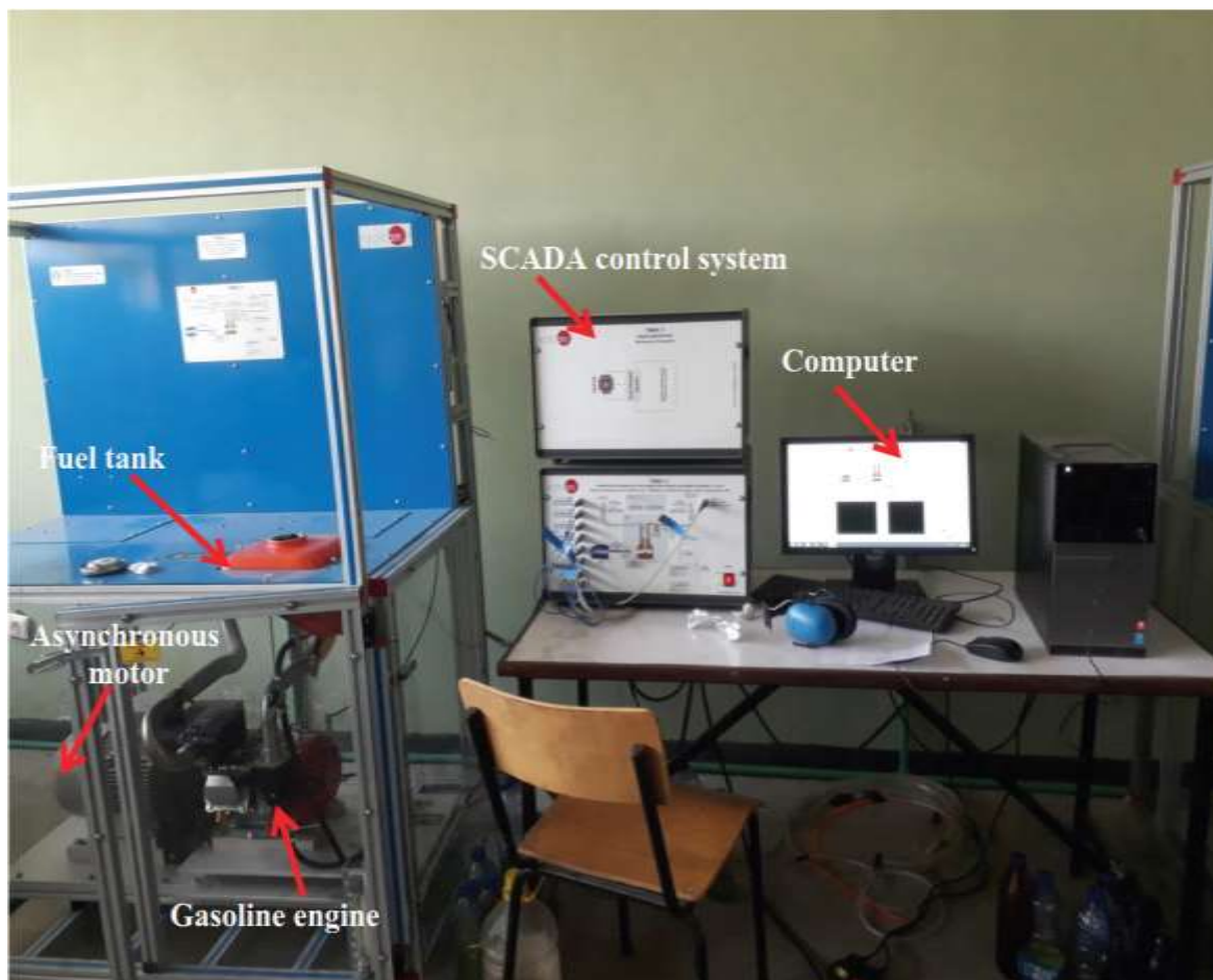
Figure 3.4 TBM3-01 engine experimental setup for SI
