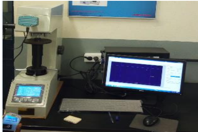
Figure 3.9 Vickers hardness testing setup [24]
