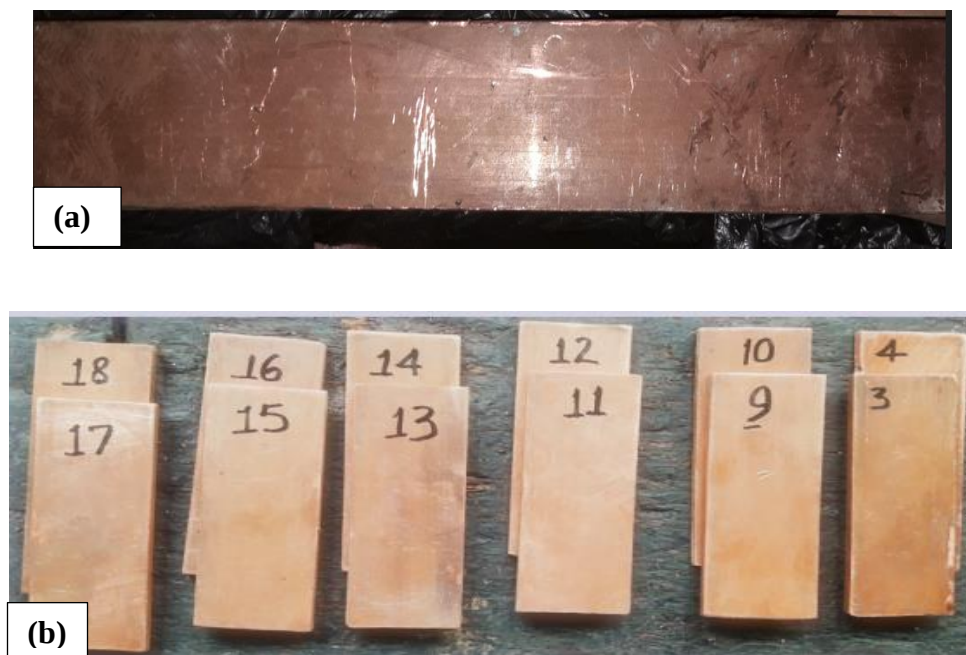
Figure 3.2 Work piece material (a) Base material stock size, (b) Copper plate samples prepared for joint formation.
