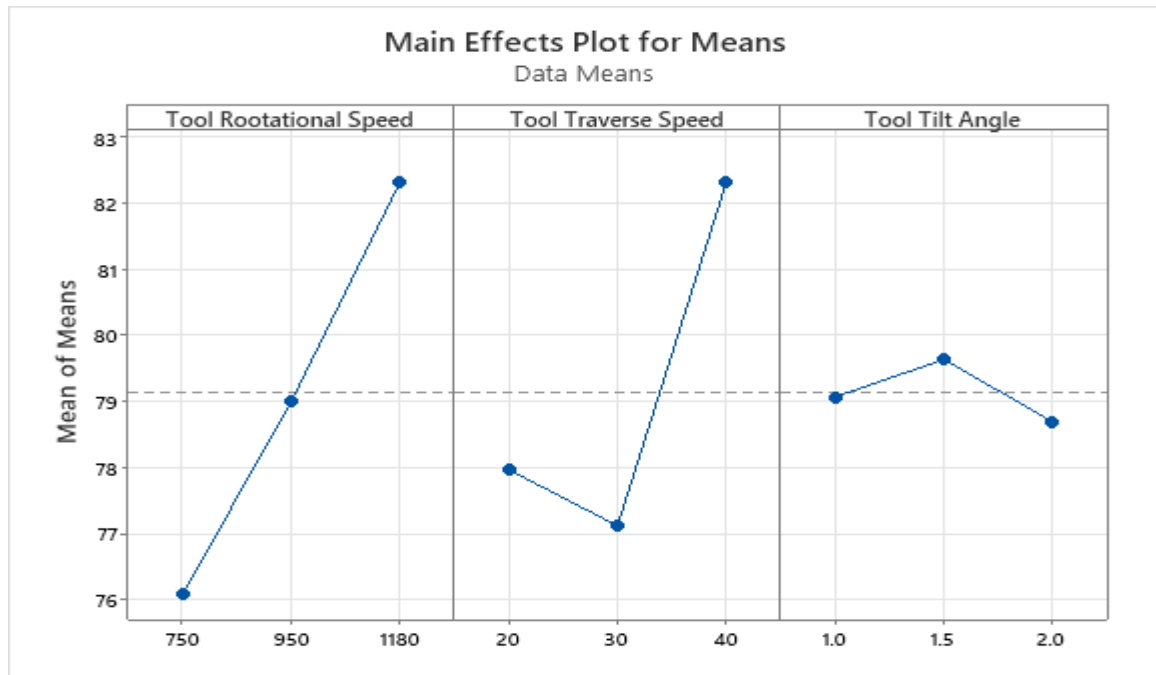
Figure 4.5 Main effect plot for means of mean hardness of FSW welded joint
