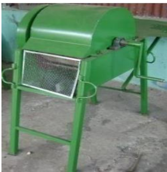
a. Manually operated maize Sheller
