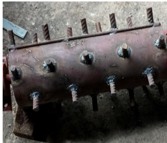
Figure 3.6. Shelling drum with spikes assembly drawing
