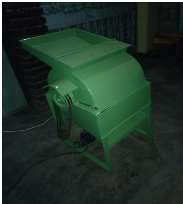
Figure 3.4. The constructed maize sheller prototype
