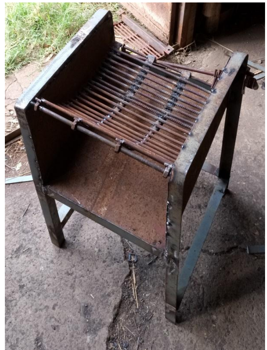
Figure 3.5. Frame of the maize sheller prototype (all dimensions in mm)
