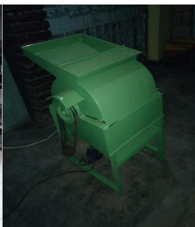
e. Motor driven maize sheller prototype
