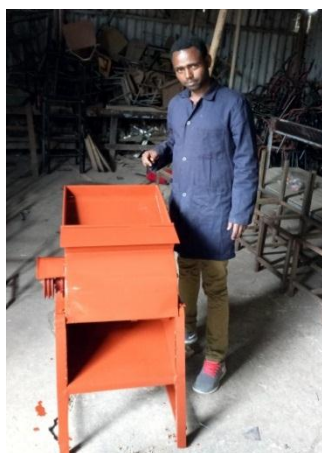
e. Motor driven maize sheller prototype
