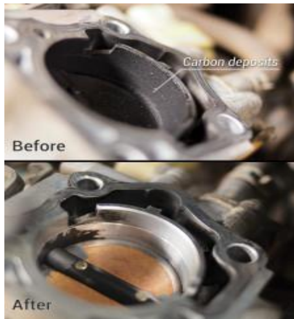
Figure 2: Coking can lead to idling problem and throttle sticking
