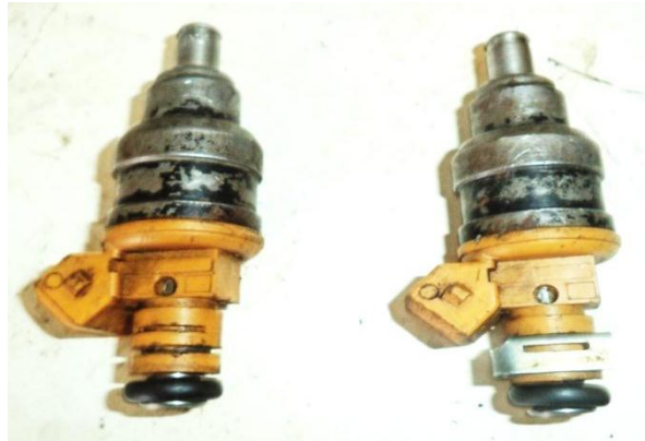
Figure 12: Photo of high-pressure injectors
