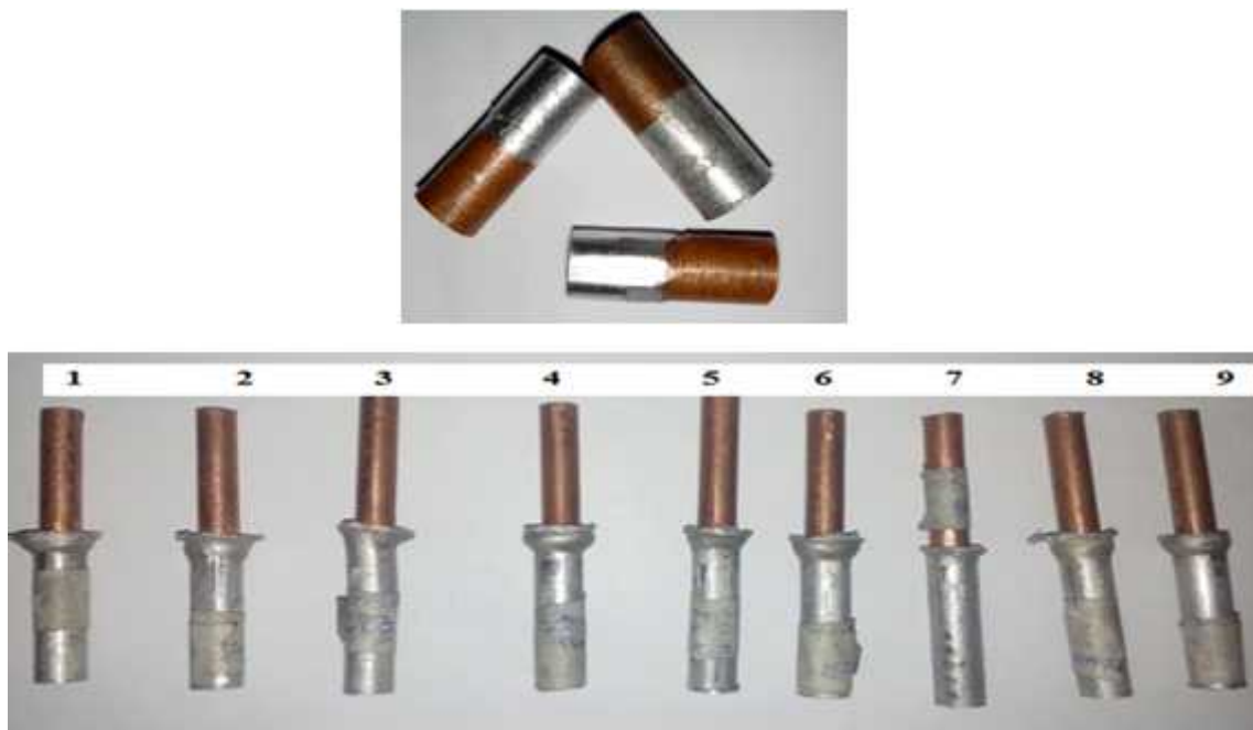
Figure 3.13 Results of nine samples friction welding of aluminium and copper from the experiment performed on the drilling machine with different parameter setting with final finished weldment
