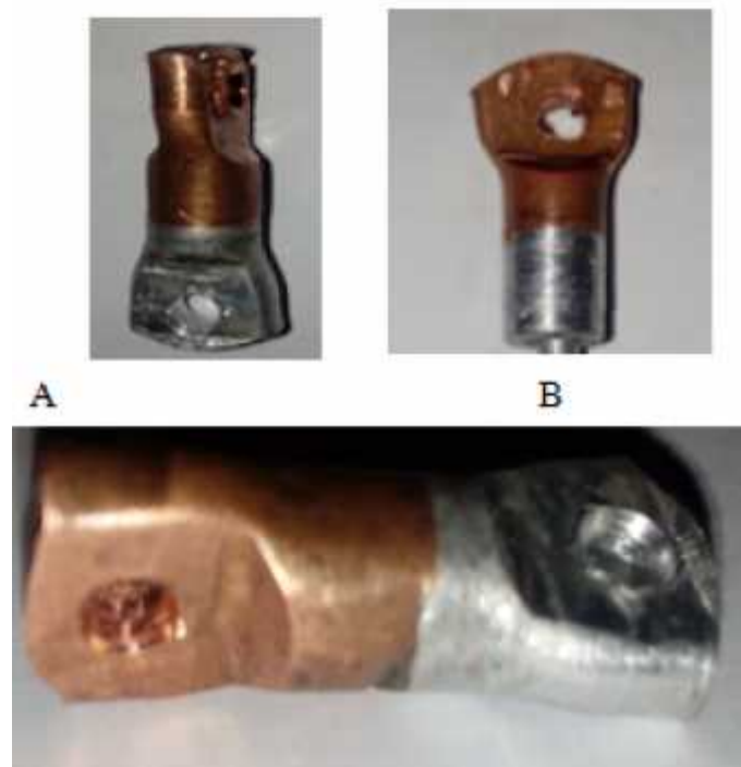
Figure 1.4 Model bimetallic connector A) Design for two side bolt and B) Design for one side bolt
