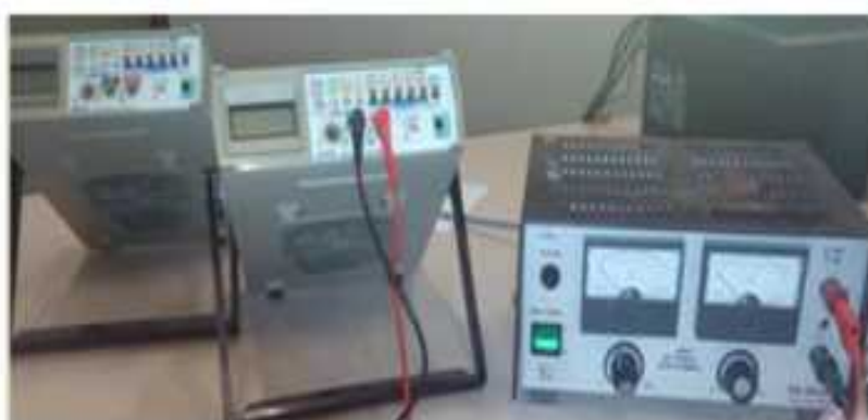
Figure 3.19 Four-probe resistance measurements assembly (Milenko, 2007)
