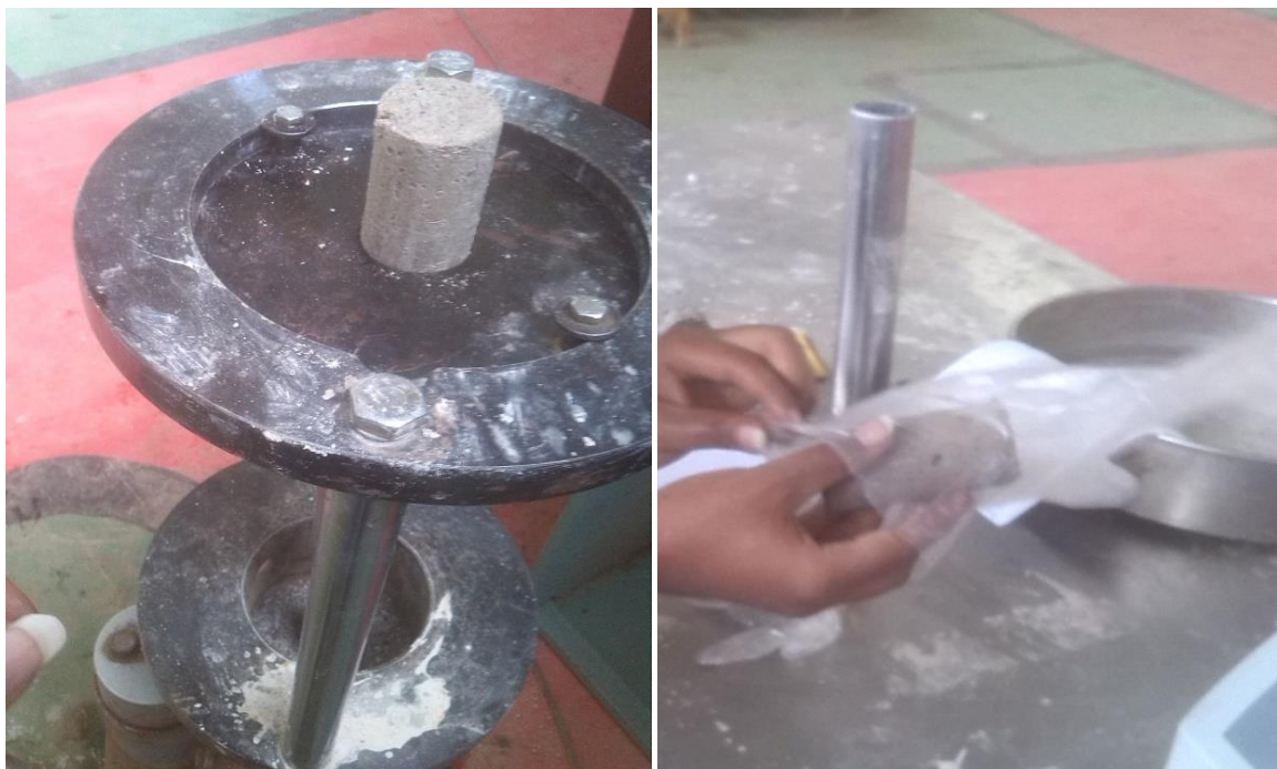
Figure B-2 Extraction of sample from the mold (left) and covering with plastic bag (right)
