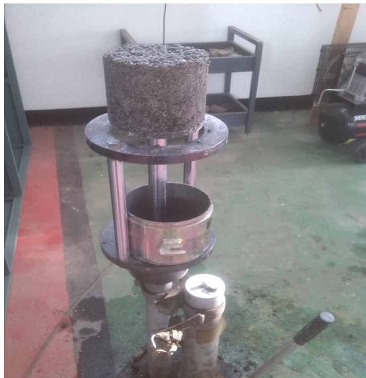
Figure C-1 During extraction of blended gravel for modified proctor test
